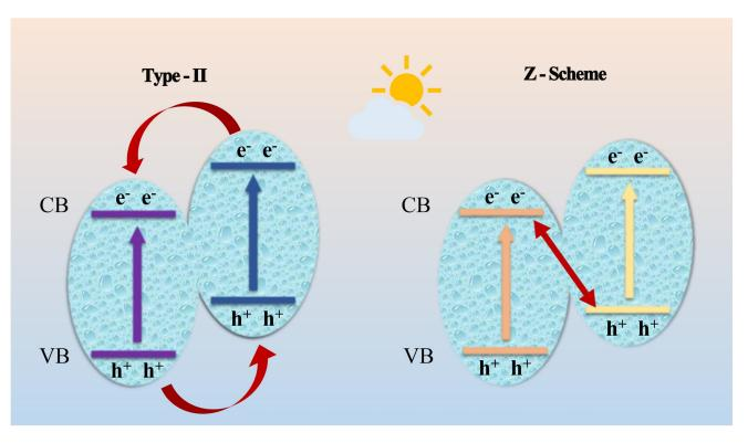
ZIS-Z and the holes remaining on the VB of pCN-N participate in the catalytic degradation of pollutants through redox reactions. Based on the capture experiments and conjectures, a conclusion can be drawn that pCN-N/ZIS-Z is a Z-scheme heterojunction.
