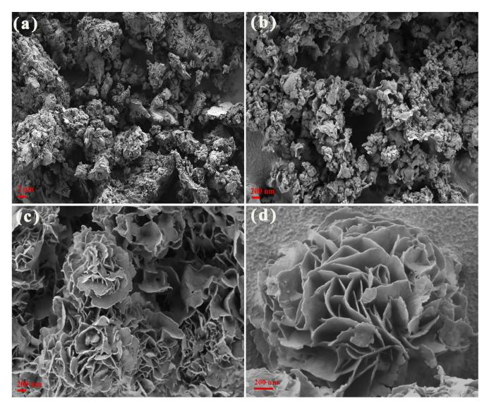
Figure 2. SEM images of bulk CN (a), pCN-N nanosheets (b), ZIS-Z nanosheets (c) and pCN-N/ZIS-Z (d).
