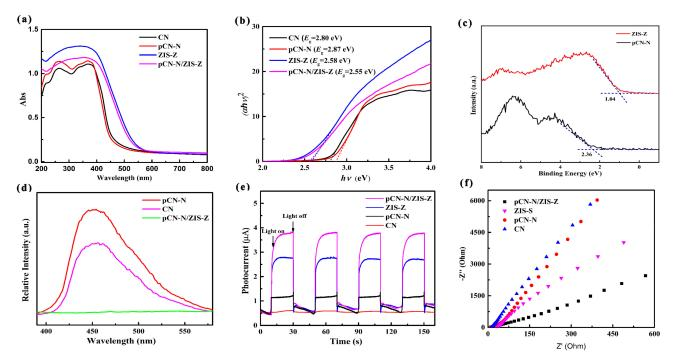
**Figure 10.** The UV–vis diffuse reflectance spectra (**a**), Plot of  $(\alpha h\nu)^2$  vs.  $h\nu$  for the bandgap energy (**b**) of different photocatalysts. XPS valence band spectra of ZIS-Z and pCN-N (**c**). The photoluminescence spectra (**d**), transient photocurrent responses (**e**), and electrochemical impedance spectroscopy (**f**) of different photocatalysts.
