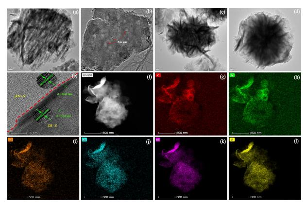
**Figure 3.** TEM images of bulk CN (**a**), pCN-N nanosheets (**b**), ZIS-Z nanosheets (**c**) pCN-N/ZIS-Z nanocomposite (**d**), HRTEM image of pCN-N/ZIS-Z nanocomposite (**e**), and elemental mapping images of pCN-N/ZIS-Z (**f**–**l**).
