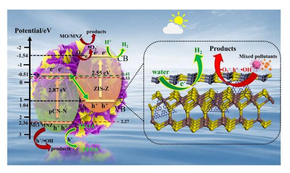
Figure 12. The possible photocatalytic mechanism of pCN-N/ZIS-Z.
