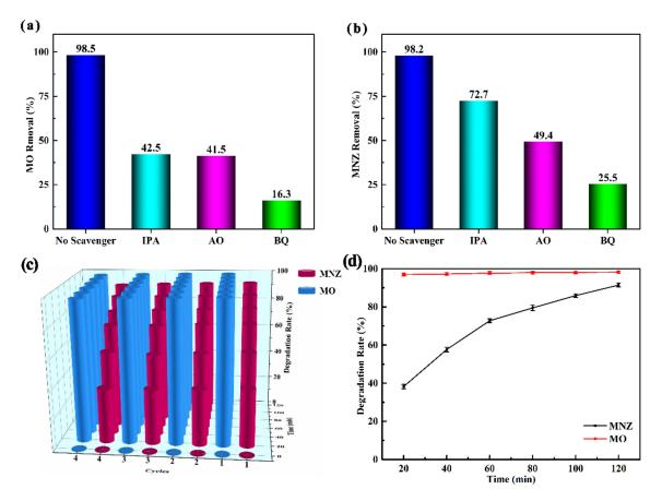
**Figure 9.** The effect of radical scavengers (IPA, AO, and BQ) on the degradation of MO (**a**) and MNZ (**b**). Photocatalytic degradation cycle (**c**) and parallel experiments (**d**) of MO/MNZ.
