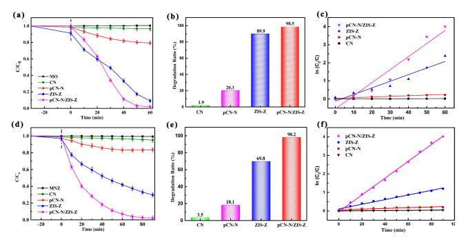
Figure 7. Photocatalytic activities of CN, pCN-N, ZIS-Z and pCN-N/ZIS-Z toward the degradation of MO (a-c), MNZ (d-f).
