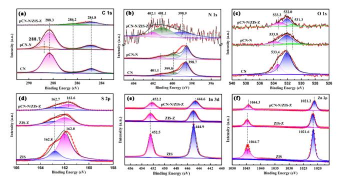
**Figure 5.** XPS spectroscopy spectra of CN, pCN-N, ZIS-Z, pCN-N/ZIS-Z nanocomposite. C 1s (**a**), N 1s (**b**), O 1s (**c**), S 2p (**d**), In 3d (**e**), and Zn 2p (**f**).
