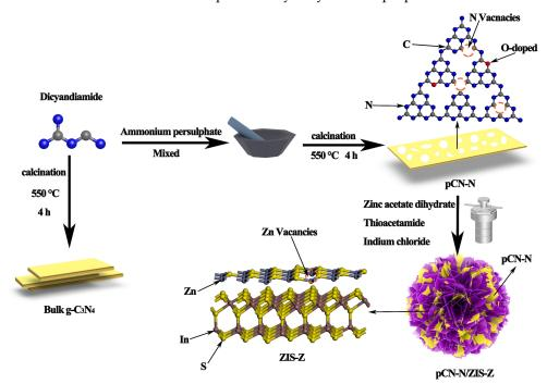
Figure 1. The synthesis process of CN, pCN-N, ZIS-Z, pCN-N/ZIS-Z.
