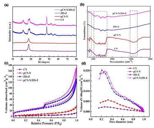
**Figure 4.** XRD patterns (**a**), FTIR spectra (**b**), surface area (**c**), and pore size distribution (**d**) of CN, pCN-N, ZIS-Z, and pCN-N/ZIS-Z catalyst.
