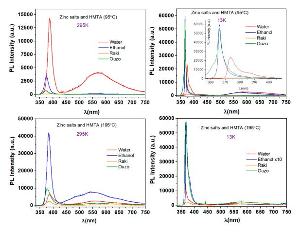
Figure 11. Typical PL spectra of samples synthesized via synthesis routes 1, 2, and 3 at 95 °C and 195 °C.
