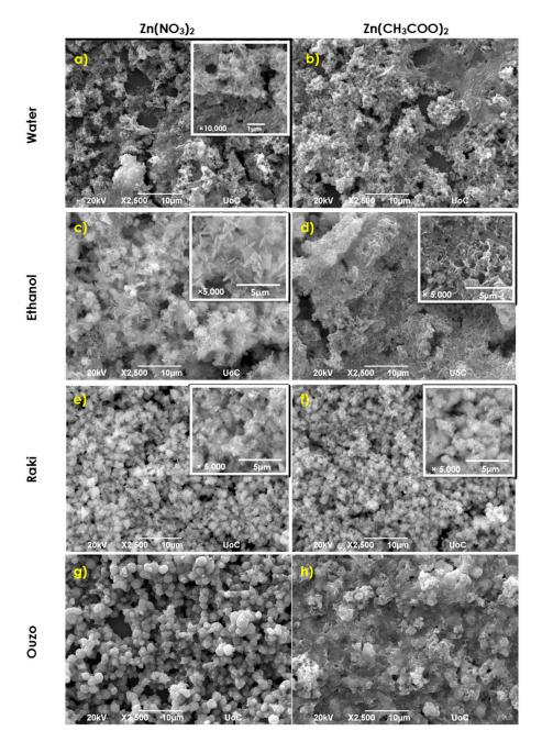
**Figure 3.** SEM images  $\times$ 2500 of ZnO samples synthesized via synthesis route 4 at 95 °C. For the case of ZnO nanostructuring zoom images are inserted.
