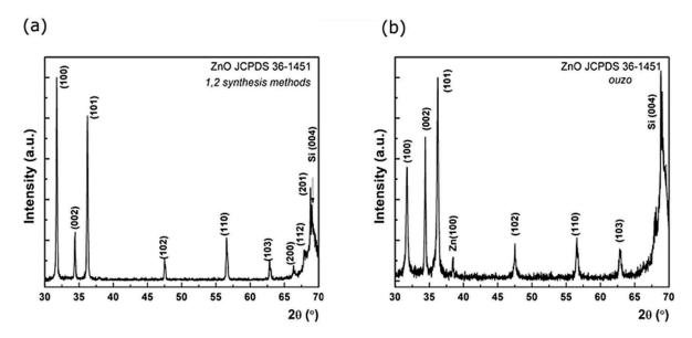
**Figure 9.** XRD spectra corresponding to the pure phase ZnO coating obtained from synthesis 2 (**a**) and to the incomplete formed ZnO phase coating obtained via synthesis 3 in Ouzo solvent (**b**).
