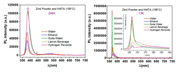
Figure 13. Typical PL spectra of samples synthesized via synthesis route 6 at 195 °C.
