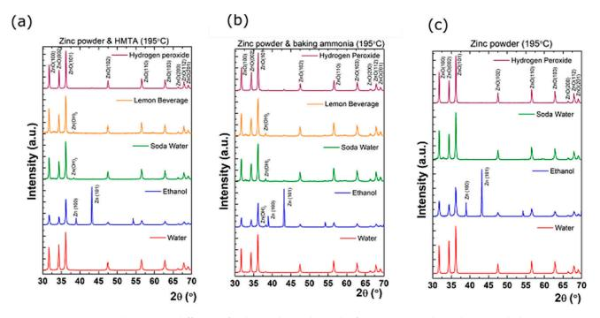
**Figure 10.** Grazing incidence X-ray diffraction for the synthesized samples from (**a**) Zn powder and Hexamethylenetetramine (HMTA), (**b**) Zn powder and baking ammonia, and (**c**) Zn powder at 195 °C in water, ethanol, soda water, lemon beverage, and hydrogen peroxide, respectively.
