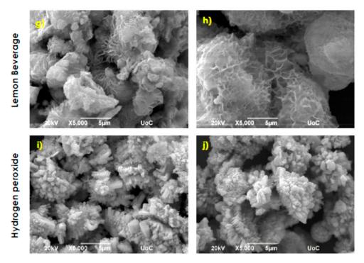
Figure 6. SEM images of ZnO samples synthesized via synthesis route 8.
