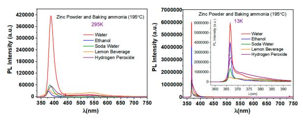
Figure 14. Typical PL spectra of samples synthesized via synthesis route 8 at 195 °C.
