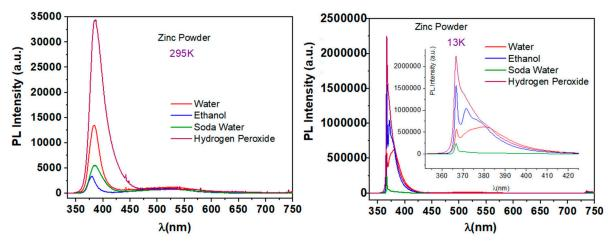
Finally, after the baking ammonia was eliminated, and syntheses were performed using the eco-friendly route 9; the obtained nanostructured ZnO materials show the PL characteristic emission spectra presented in Figure 15.
