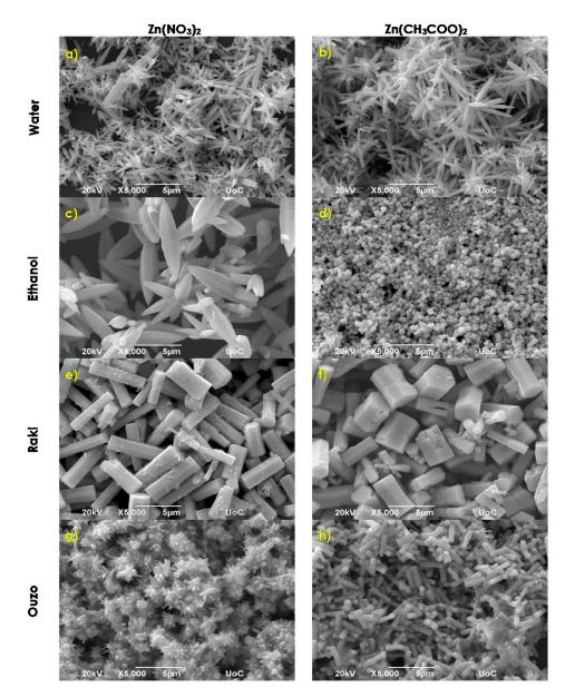
Figure 2. SEM images of ZnO samples synthesized via synthesis routes 1, 2, and 3 at 195 °C.
