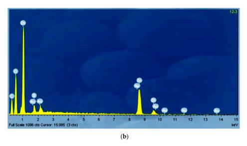
**Figure 8.** Typical EDX spectra of (**a**) ZnO samples synthesized with zinc nitrate and HMTA at 195 °C in ethanol solvent on Si(100) substrate and (**b**) ZnO samples synthesized with zinc acetate and HMTA at 95 °C in Ouzo solvent on Si(100) substrate.
