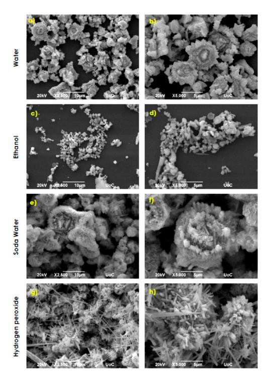
**Figure 7.** SEM images of ZnO samples synthesized via synthesis route 9 at 195 °C (a,b) two different magnifications for samples grown in water, (c,d) two different magnifications for samples grown in ethanol, (e,f) two different magnifications for samples grown in soda water (g,h) two different magnifications for samples grown in hydrogen peroxide.
