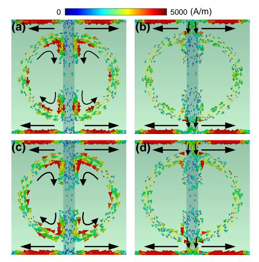
and the graphene patch. As the graphene Fermi level increases, the surface currents along the graphene patch become stronger.
