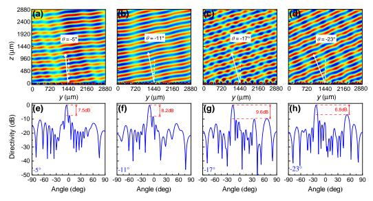
**Figure 6.** (**a**–**d**) Near-field electric field distributions  $|E_x|$  and (**e**–**h**) far-field directivity for deflected reflection angles of (**a**,**e**)  $\theta = -5^\circ$ ; (**b**,**f**)  $-11^\circ$ ; (**c**,**g**)  $-17^\circ$ ; and (**d**,**h**)  $-23^\circ$ .
