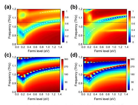
**Figure 4.** Simulated reflection (**a**,**b**) amplitude and (**c**,**d**) phase spectra for different graphene Fermi levels. The calculations were performed with (**a**,**c**)  $t = 40 \ \mu\text{m}$  and (**b**,**d**)  $t = 50 \ \mu\text{m}$ , respectively.
