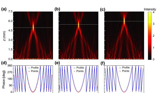
**Figure 8.** (**a**–**c**) Electric field intensity distributions  $|E_x|^2$ , (**d**–**f**) desired phase profiles (blue curves) and discrete phase points of the focusing metasurface array with designed focal lengths of (a,d) F = 5 mm, (**b**,**e**) 5.5 mm and (**c**,**f**) 6 mm operating at 1.05 THz.
