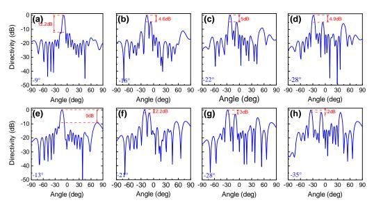
**Figure 7.** Far-field directivity for the deflected reflection angle of (**a**,**e**)  $\theta = -5^{\circ}$ ; (**b**,**f**)  $\theta = -11^{\circ}$ ; (**c**,**g**)  $\theta = -17^{\circ}$ ; (**d**,**h**)  $\theta = -23^{\circ}$  under oblique incident angles of (**a**–**d**)  $5^{\circ}$ ; and (**e**–**f**)  $10^{\circ}$ .
