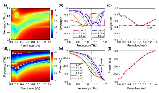
**Figure 2.** Simulated reflection (**a**,**b**) amplitude and (**d**,**e**) phase spectra for different graphene Fermi levels. Reflection (**c**) amplitude and (**f**) phase as functions of the graphene Fermi level at 1.05 THz.
