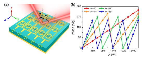
**Figure 5.** (a) Schematic of the phased array structure for achieving dynamic reflection beam steering; (b) reflection phase distributions of the designed phased array for achieving four specific deflection angles.
