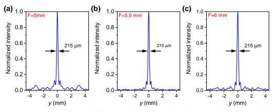
Figure 9. Normalised electric field intensity along y axis (when z locates at the focal points) for (a) F = 5 mm, (b) 5.5 mm and (c) 6 mm, respectively.
