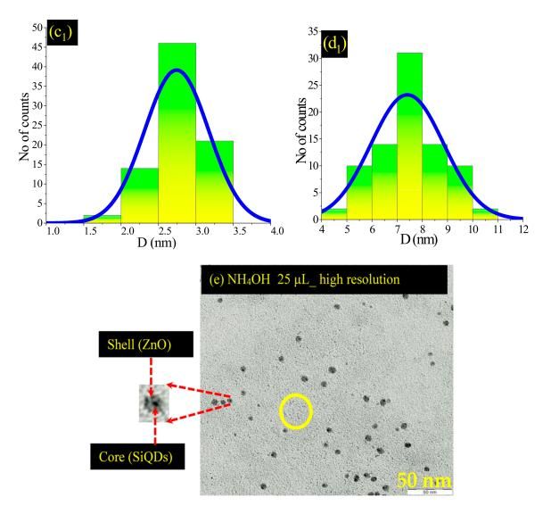
**Figure 7.** (**a**–**d**) EFTEM images of the colloidal ZnSiQD suspension in acetone prepared with NH<sub>4</sub>OH of 0, 15, 20, and 25  $\mu$ L, respectively. (**a**<sub>1</sub>–**d**<sub>1</sub>) particle size distributions of the colloidal ZnSiQDs (20 mL) suspended in acetone with NH<sub>4</sub>OH of 0, 15, 20, and 25  $\mu$ L, respectively. (**e**) NH<sub>4</sub>OH: 25  $\mu$ L high resolution.
