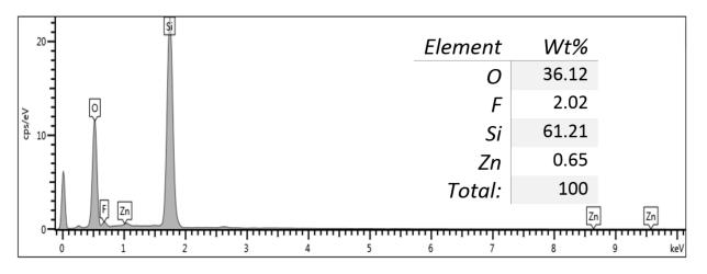
Figure 6. EDX images of the prepared ZnPSi with 0.17 g of included Zn.
