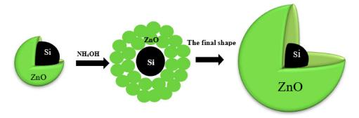
Figure 14. The schematic diagram for the mechanism of NH<sub>4</sub>OH influence on the ZnO shell.
