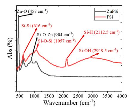
Figure 4. FTIR spectra of Psi and ZnPSi.
