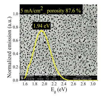
Figure 2. FESEM morphology combined with PL of the PSi etched at 5 mA/cm<sup>2</sup>.
