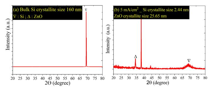
Figure 3. XRD analysis for (a) bulk Si; (b) ZnPSi at etching current density of 5 mA/cm<sup>2</sup>.
