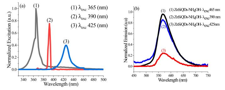
**Figure 12.** (a) Excitation spectra of source at excitation peak of (1) 365 nm, (2) 390 nm, and (3) 425 nm. (b) PL spectra of the colloidal ZnSiQD suspension in acetone containing 25  $\mu$ L of NH<sub>4</sub>OH excited at the wavelengths of (1) 365 nm, (2) 390 nm, and (3) 425 nm.
