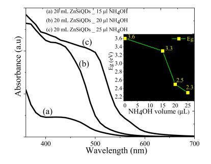
**Figure 13.** UV–vis absorbance of the colloidal ZnSiQD suspension in acetone synthesized with NH<sub>4</sub>OH of (**a**) 15  $\mu$ L (**b**), 20  $\mu$ L, and (**c**) 25  $\mu$ L.
