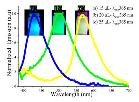
**Figure 11.** PL spectra (excited at 365 nm) of the colloidal ZnSiQDs synthesized with NH<sub>4</sub>OH of (a) 15  $\mu$ L, (b) 20  $\mu$ L, and (c) 25  $\mu$ L.
