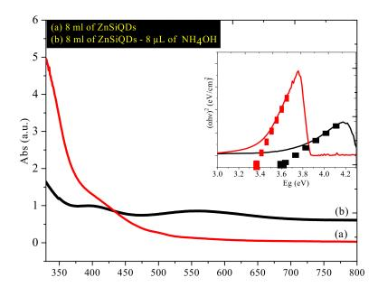
**Figure 9.** ZnSiQD suspension in acetone prepared (**a**) without and (**b**) with NH4OH (Inset: Tauc plot for the bandgap estimation.
