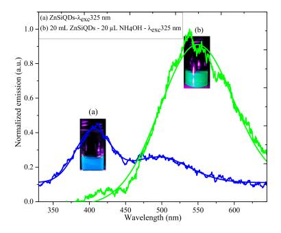
**Figure 10.** PL spectra (excited at 325 nm) of the colloidal ZnSiQD suspension in acetone synthesized (**a**) without and (**b**) with  $NH_4OH$  (20  $\mu$ L). The bottles in the inset show the corresponding blue and green visible fluorescence observed by the naked eyes.
