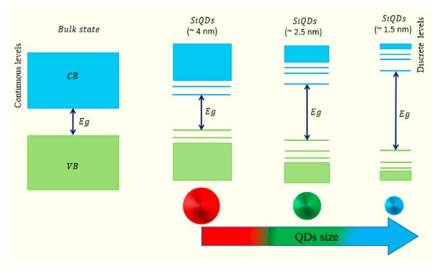
Figure 1. Schematic depiction of how the change from the bulk to the QDs impact the CB, VB levels, and Eg in QDs.
