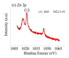
Figure 5. The XPS profile of the ZnPSi for (a) Si2p (103.5 eV), (b) O1s (532.84 eV), and (c) Zn2p (1022.3 eV).
