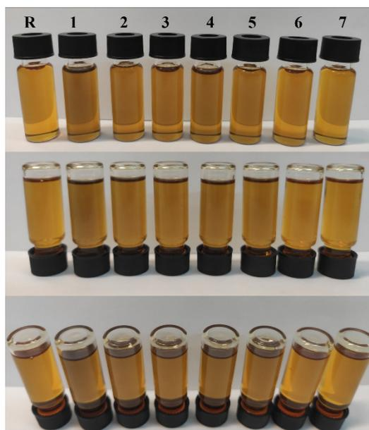
**Figure 1.** Photographs of the reference 5W-40 synthetic oil (R) and the prepared oil samples incorporating rGO at different concentrations (R—0 wt %, 1—0.2 wt %, 2—0.1 wt %, 3—0.08 wt %, 4—0.06 wt %, 5—0.04 wt %, 6—0.02 wt % and 7—0.01 wt %), photographed from different angles.
