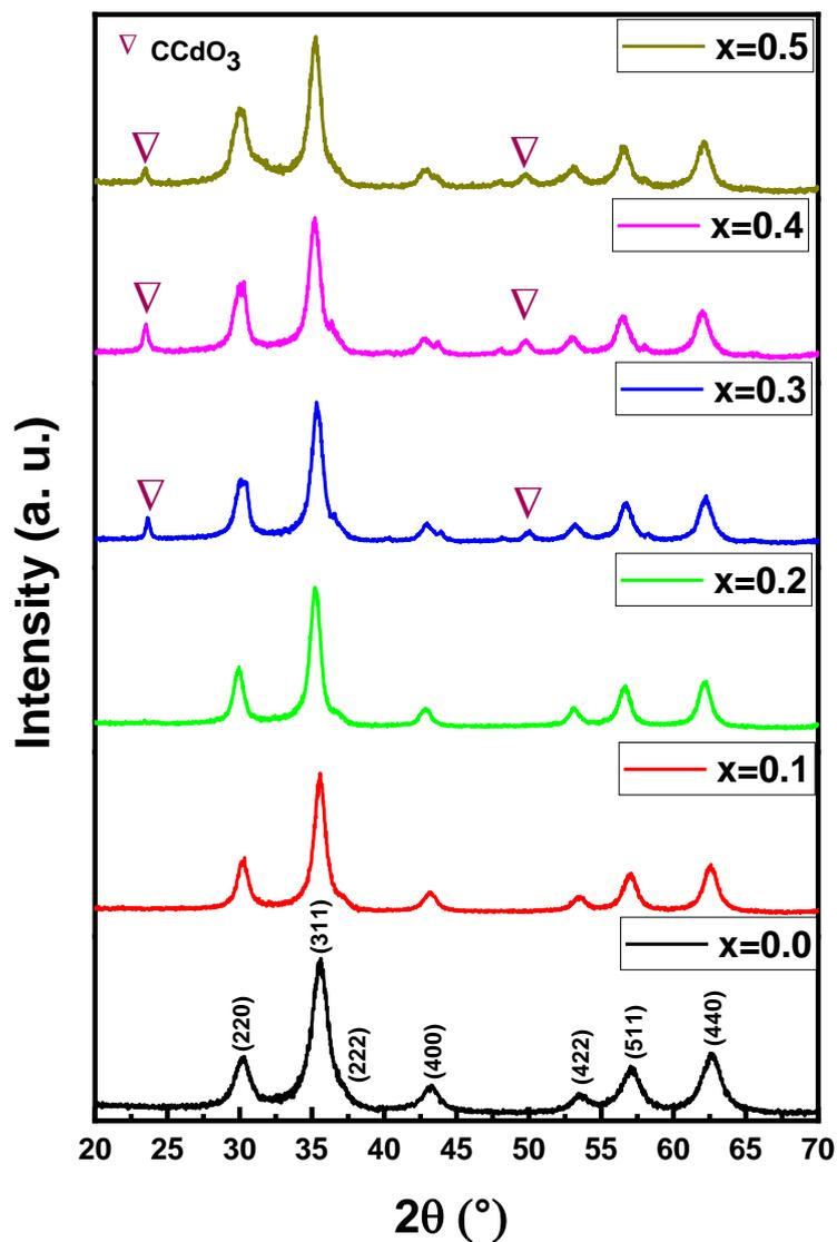
Figure 1. XRD powder patterns of  $(\text{Mn}_{0.5}\text{Zn}_{0.5})[\text{Cd}_x\text{Fe}_{2-x}]\text{O}_4$  ( $x \leq 0.05$ ) NSF.
