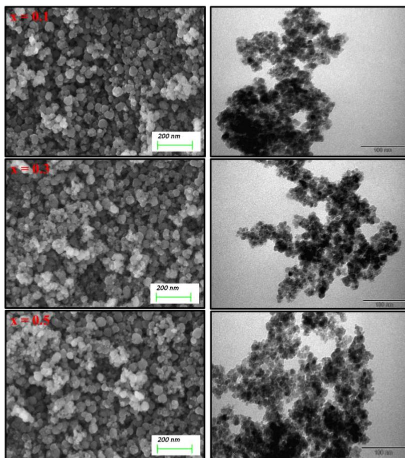
Figure 2. SEM and TEM images of  $(\text{Mn}_{0.5}\text{Zn}_{0.5})[\text{Cd}_x\text{Fe}_{2-x}]\text{O}_4$  ( $x = 0.1, 0.3$  and  $0.5$ ) NSFs.
