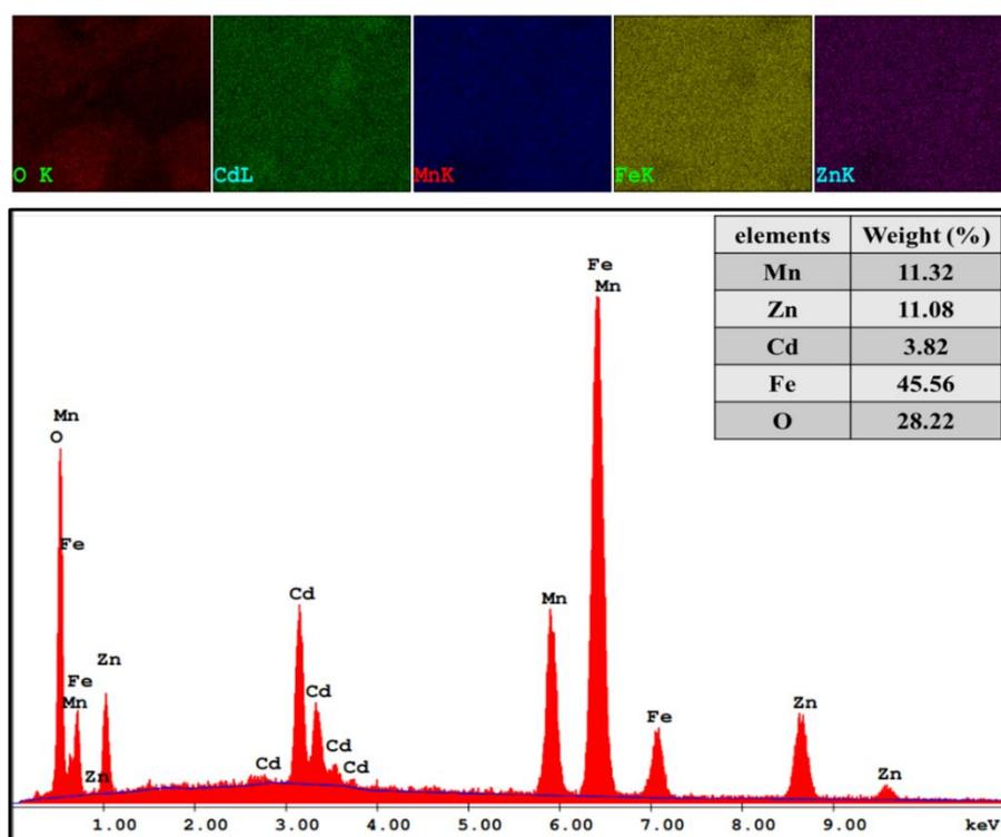
Figure 3. EDX and elemental mapping of  $(\text{Mn}_{0.5}\text{Zn}_{0.5})[\text{Cd}_x\text{Fe}_{2-x}]\text{O}_4$  ( $x = 0.2$ ) NSFs.
