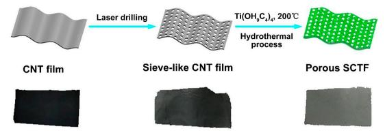
**Figure 1.** The schematic procedure of fabricating sieve-like carbon nanotube (CNT)/TiO2 nanowire film (SCTF) and the corresponding films obtained at each step.
