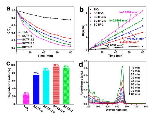
**Figure 4.** Photocatalytic degradation curves (**a**), kinetic curves (**b**) and degradation ratios (**c**) of RhB for different photocatalysts under simulated solar irradiation. (**d**) Absorption spectra of RhB with SCTF-2.5 as photocatalyst in different reaction times under simulated solar irradiation.
