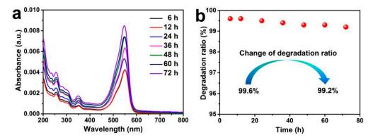
**Figure 6.** UV-vis spectra (**a**) and the degradation ratios (**b**) of the RhB solution for different times during the continuous-flow photodegradation under simulated solar irradiation.
