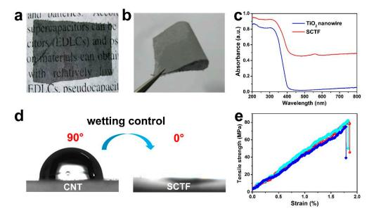
**Figure 2.** (**a**,**b**) Digital photographs of SCTF. (**c**) UV-vis DRS of a TiO<sub>2</sub> nanowire and SCTF. (**d**) Photograph of a water droplet standing on a sieve-like CNT film and SCTF. (**e**) Tensile stress–strain curves of SCTFs.
