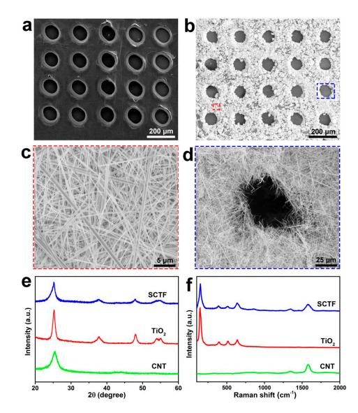
**Figure 3.** SEM images of a sieve-like CNT film (**a**) and SCTF at low and high magnifications (**b**–**d**). XRD patterns (**e**) and Raman spectra (**f**) of CNT, TiO<sub>2</sub> and SCTF.
