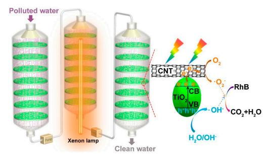
**Figure 5.** Schematic diagram of the continuous-flow photodegradation and photocatalytic degradation mechanism of RhB on SCTF-2.5.
