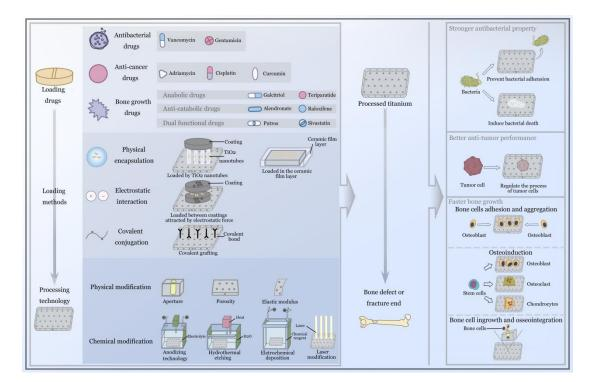
**Figure 1.** Schematical presentation of local drug delivery system on a titanium implant modified by metal processing technology, and the excellent advantages after implantation.
