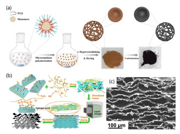
**Figure 3.** Fabrication of carbon aerogels: (a) Powdery carbon aerogels. Reprinted with permission from Ref. [41], Copyright 2017, Elsevier Ltd. (b,c) 2D titanium carbide and bacterial cellulose-derived carbon aerogels. (b) fabrication process and (c) SEM image of the carbon aerogels. Reprinted with permission from Ref. [43], Copyright 2019, American Chemical Society.
