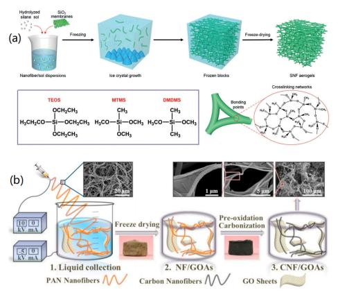
**Figure 1.** Fabrication of aerogels: (a) Freezing-mediated growth and freeze-drying fabrication of SNF aerogels. Reprinted with permission from Ref. [20], Copyright 2020, Wiley VCH. (b) Electrospinning and freeze-drying promoted fabrication of CNF/GO hybrid aerogels. Reprinted with permission from Ref. [21], Copyright 2019, Elsevier.
