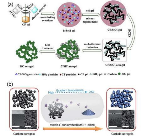
**Figure 7.** Fabrication of carbide-based aerogels: (a) SiC aerogels. Reprinted with permission from Ref. [67], Copyright 2019, Elsevier Ltd. (b) TiC and NbC aerogels. Reprinted with permission from Ref. [68], Copyright 2015, Royal Society of Chemistry.
