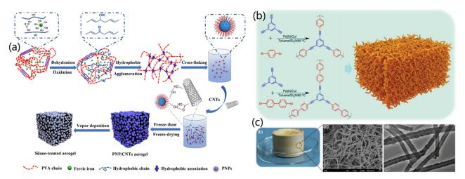
**Figure 4.** Fabrication of CNT-based aerogels: (a) PVA-based nanoparticles (PNP)/CNTs aerogels. Reprinted with permission from Ref. [47], Copyright 2020, Elsevier Ltd., (b,c) Hollow CNT aerogels: (b) synthesis process and (c) photograph and microscopy characterizations. Reprinted with permission from Ref. [6], Copyright 2019, Wiley VCH.
