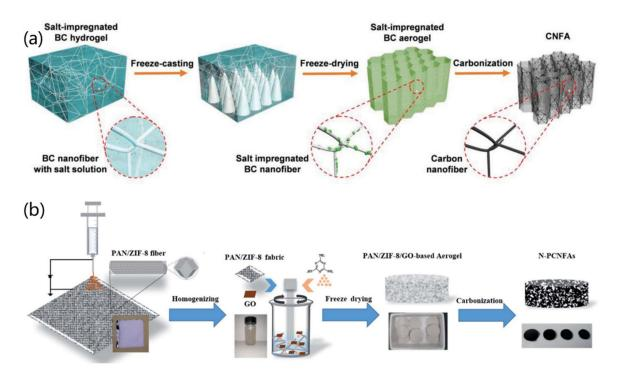
**Figure 5.** Fabrication of CNF-based aerogels: (a) BC nanofiber-based fabrication of CNF aerogels. Reprinted with permission from Ref. [56], Copyright 2020, Wiley VCH. (b) Electrospinning, freeze drying, and carbonization-based formation of CNF aerogels. Reprinted with permission from Ref. [59], Copyright 2020, Royal Society of Chemistry.
