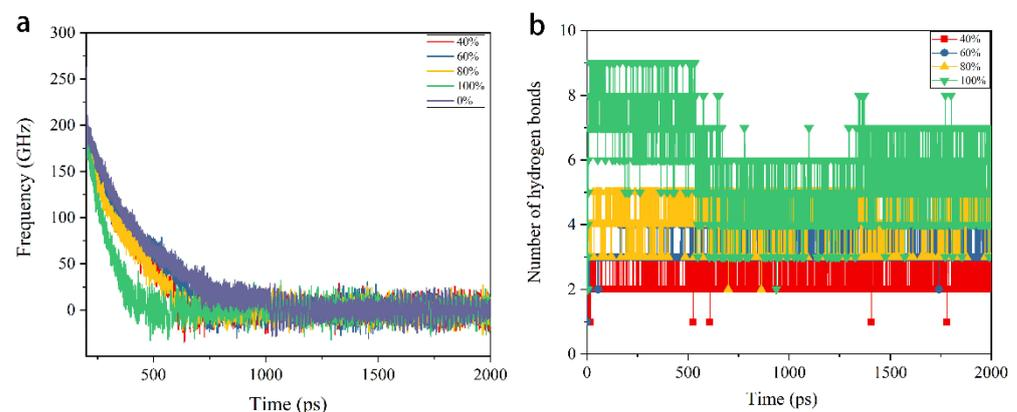
**Figure 3.** (a) The rotation frequency of rotor during braking process when pristine CNTs, CNTs with 40%, 60%, 80%, 100% grafted hydroxyl groups are applied. (b) The number of hydrogen bonds when 40%, 60%, 80%, 100% hydroxyl groups are grafted, respectively.
