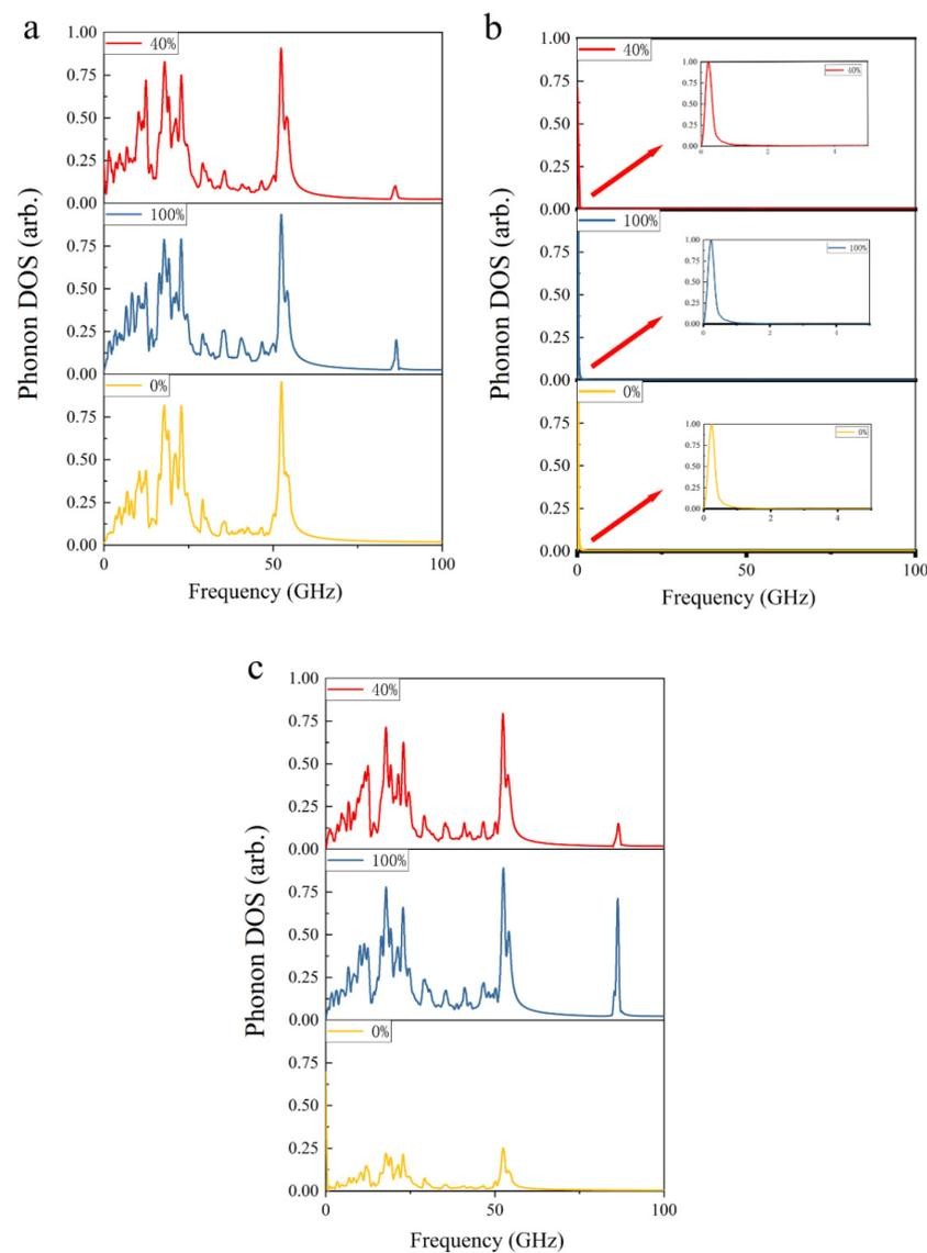
**Figure 4.** The phonon DOS of the transmission system in three stages when pristine carbon nanotubes, carbon nanotubes grafted with 40% and 100% hydroxyl groups are applied, respectively: (a) relaxation, (b) acceleration, and (c) deceleration.
