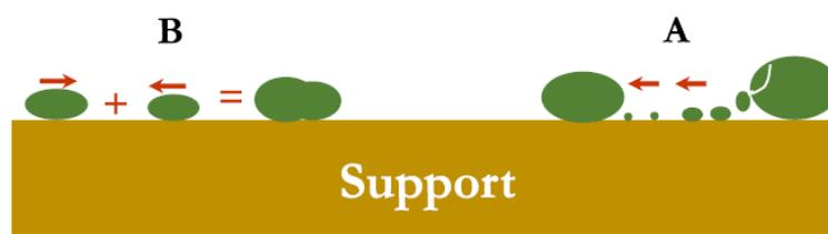
**Figure 7.** Sintering pathways of catalysts via crystal growth by (A) atomic migration and (B) crystallite migration. Reprinted with permission from Ref. [30]. Copyright 2019 Elsevier.
