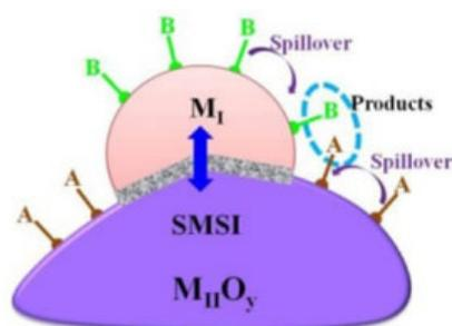
**Figure 15.** Spillover: an example of the bifunctional effect caused by SMSI. Reprinted with permission from Ref. [128]. Copyright 2017 Elsevier.
