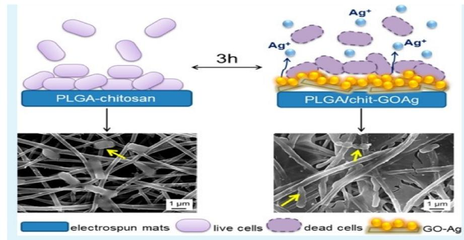
**Figure 11.** Preparation process of electrospun biopolymer nanofiber mats functionalized with graphene oxide-silver nanocomposites [73] Adapted with permission from Ref. [73]. 2015, American Chemical Society.
