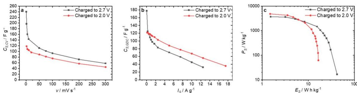
**Figure 6.** Electrochemical measurements on the ACF, which was activated twice (CO<sub>2</sub> and H<sub>2</sub>O):  $C_{S,CV}$  at different scan rates  $\nu$  (a),  $C_{S,GDC}$  at different current densities  $I_S$  per electrode (b), and Ragone plot calculated from GDC for the whole device (c). The values in black were obtained for charging the EDLC to 2.7 V, and those in red for charging to 2.0 V.
