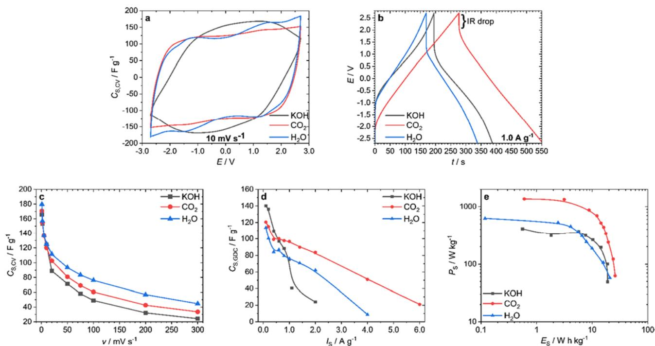
**Figure 2.** Electrochemical measurements of the EDLCs: CVs at a scan rate  $\nu$  of 10 mV s<sup>-1</sup> (a), GDC at a specific current  $I_s$  of 1.0 A g<sup>-1</sup> (b),  $C_{s,cv}$  at different scan rates  $\nu$  (c),  $C_{s,gdc}$  at different current densities  $I_s$  (d), and Ragone plot calculated from GDC per device (e).
