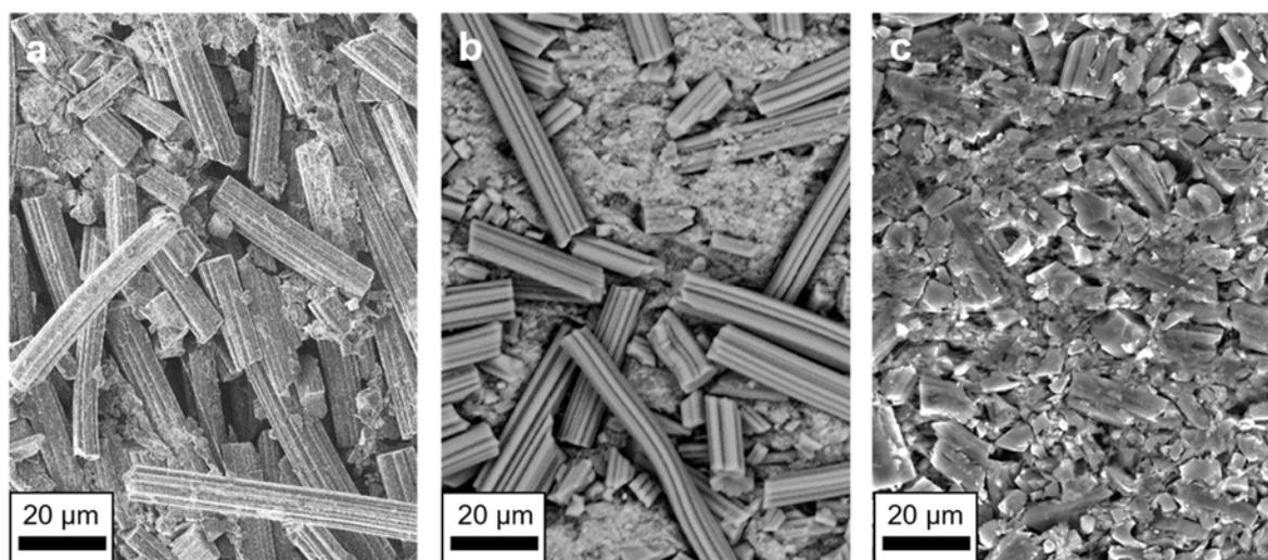
**Figure 3.** SEM micrographs of the electrode produced from the ACFs activated with CO<sub>2</sub> (a), H<sub>2</sub>O (b), and KOH (c).
