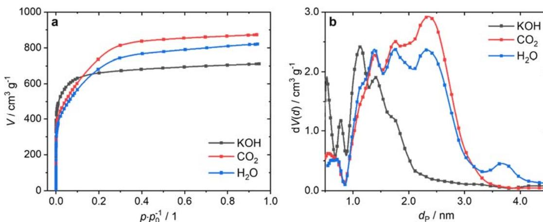
**Figure 1.** Isotherms (a) and PSDs (b) of the ACFs activated with KOH,  $\text{CO}_2$ , and  $\text{H}_2\text{O}$  ( $\text{N}_2$ ; 77 K; NLDFT; slit-pore model).
