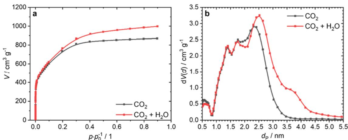
**Figure 5.** Isotherms (a) and PSDs (b) of the ACFs activated with CO<sub>2</sub>, and with CO<sub>2</sub> followed by H<sub>2</sub>O (N<sub>2</sub>; 77 K; NLDFT; slit-pore model).
