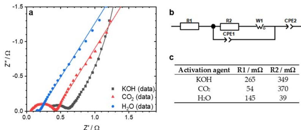
**Figure 4.** Nyquist plot of the EIS measurements (a). The symbols indicate the actual data measured; the lines represent the fit to the equivalent circuit, shown in (b). The table in (c) shows the values for resistors R1 and R2 determined by the fit.
