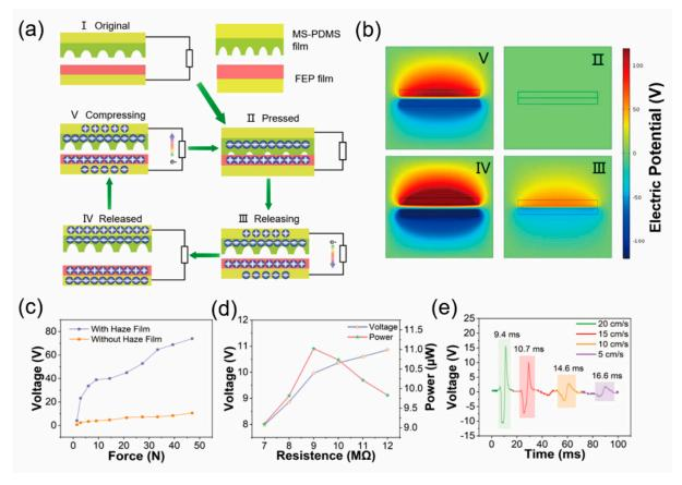
**Figure 2.** (a) Working principle of the MS-TENG; (b) FEA simulation of the MS-TENG electric potential distribution; (c) peak voltage of MS-TENG and without microstructure TENG under variable applied force from 0 to 50 N; (d) the output performance of MS-TENG under different load resistances; (e) the voltage wave of MS-TENG under speed of 5, 10, 15, and 20 cm/s.
