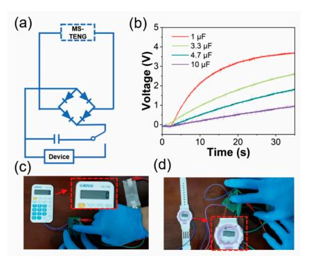
**Figure 5.** (a) The equivalent circuit of a self-powered system; (b) charging voltage of different capacitor which is charged by MS-TENG; (c) powering for an electronic calculator; (d) powering for an electronic watch.
