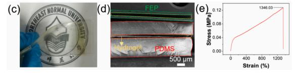
**Figure 1.** (a) The application scenarios of MS-TENG; (b) the fabricating process of the MS-TENG; (c) the optical image of MS-TENG at bending state; (d) the SEM image of the MS-PDMS; (e) tensile strength testing of hydrogel.
