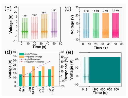
**Figure 3.** (a) MS-TENG monitors the body joint motion system; (b) outputting triboelectric voltage of MS-TENG at different bend angles; (c) outputting triboelectric voltage of MS-TENG at different frequencies; (d) response of output triboelectric voltage of MS-TENG at different bending angles and frequencies; (e) durability property of MS-TENG.
