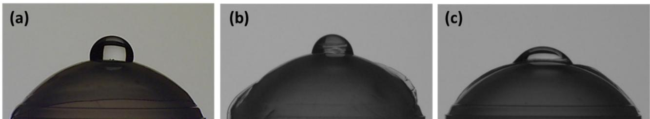
**Figure 6.** Water contact angle photographs of (a) the standard, (b) the LPMSN–siloxane, and (c) the LPMSN–amine CLs after HA soaking, respectively.
