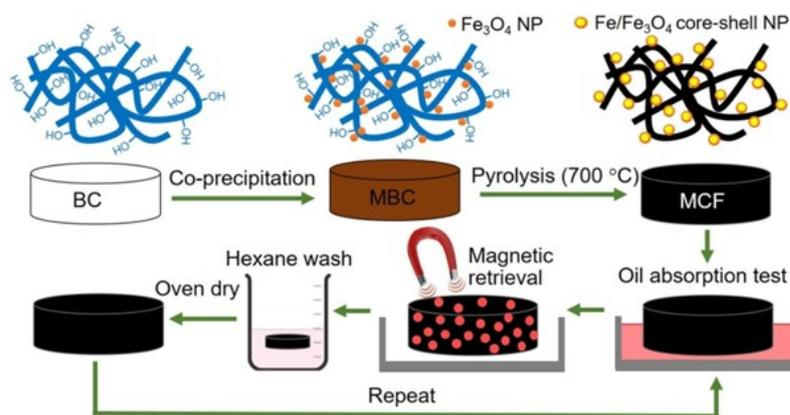
**Figure 13.** A diagram for the synthesis of magnetic carbon fiber (MCF) aerogels and the oil absorption measurement. Reproduced with permission [165]. Copyright 2020, American Chemical Society.
