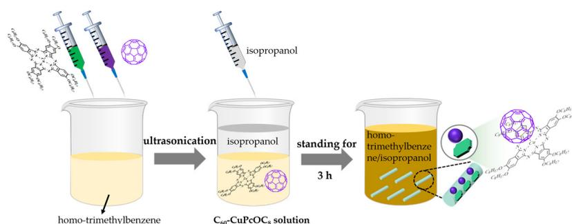
**Scheme 2.** Illustration of preparation process of C<sub>60</sub>-CuPcOC<sub>8</sub> assembly through the liquid–liquid interface deposition method.
