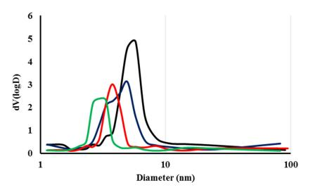
**Figure S2.** Pore size distribution of MSNs (**black**), AlClPc-MSNs (**blue**), cisplatin-MSNs (**red**) and AlClPc/cisplatin-MSNs (**green**).
