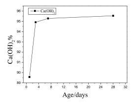
**Figure 5.** The mass loss of Ca(OH)<sub>2</sub> at different ages.
