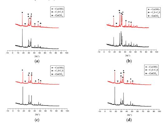
**Figure 8.** XRD patterns of cement pastes with 3% or without of nano-SiO<sub>2</sub> at different ages: (a) one day; (b) three days; (c) seven days; and (d) 28 days.
