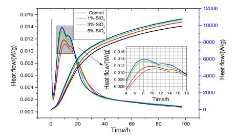
Figure 7. Effect of nano-SiO<sub>2</sub> on cement hydration exothermic rate and hydration heat.
