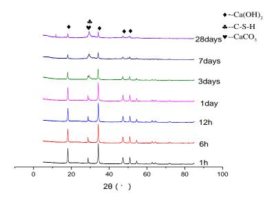
**Figure 3.** XRD patterns of the reaction of nano-SiO<sub>2</sub> with Ca(OH)<sub>2</sub>.
