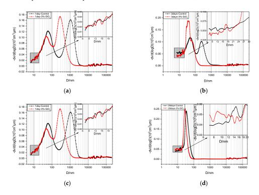
**Figure 12.** Pore size distribution of cement pastes with 3% or without nano-SiO<sub>2</sub> at different ages: (a) 1 day; (b) 3 days; (c) 7 days; and (d) 28 days.
