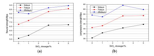
**Figure 6.** Flexural and compressive strength of cement contained Nano-SiO<sub>2</sub>. (a) Flexural strength; and (b) compressive strength.
