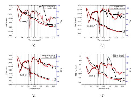
**Figure 9.** TG-DSC curves of cement pastes with 3% or without of nano-SiO<sub>2</sub> at different ages: (a) 1 day; (b) 3 days; (c) 7 days; and (d) 28 days.
