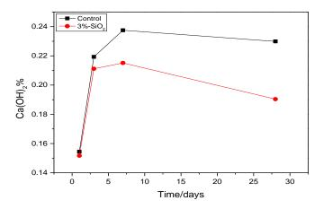
**Figure 10.** The mass loss of Ca(OH)<sub>2</sub> at difference ages.
