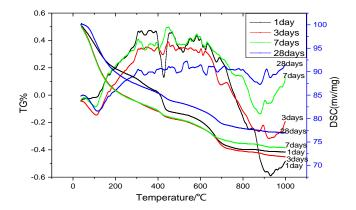
**Figure 4.** Thermogravimetric-differential scanning calorimetry (TG-DSC) curves of the products of the reaction of nano-SiO<sub>2</sub> with Ca(OH)<sub>2</sub>.
