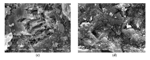
**Figure 11.** SEM images: (a) control cement at three days (b) cement with nano-SiO<sub>2</sub> 3% at three days (c) control cement at 28 days; and (d) cement with nano-SiO<sub>2</sub> 3% at 28 days.
