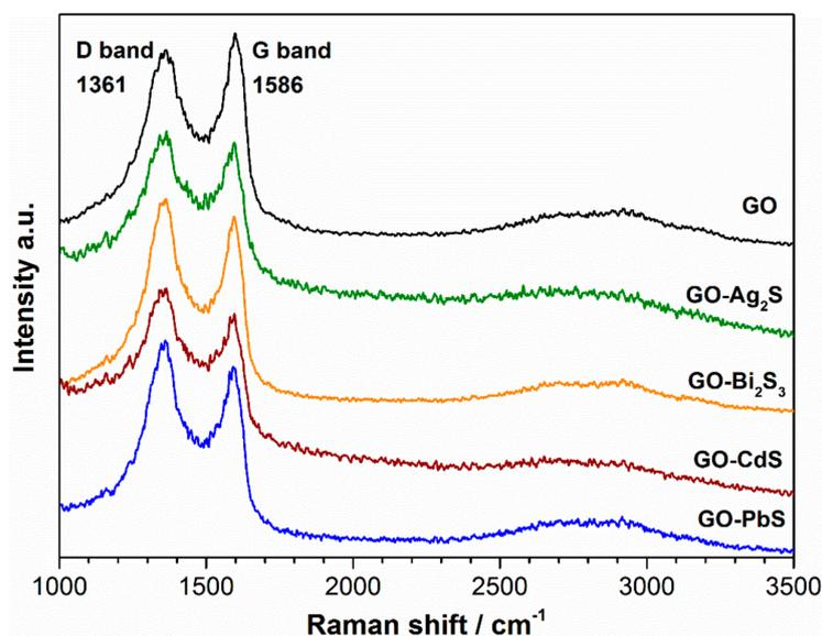
**Figure 6.** Raman spectra of graphene oxide and derived hybrids having the indicated metal sulfides (1000–3500  $\text{cm}^{-1}$  region).
