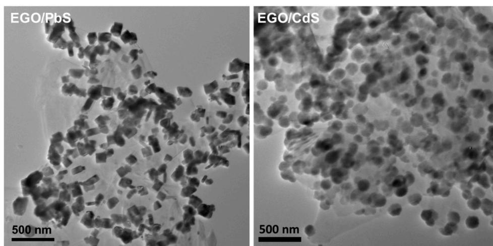
**Figure 8.** Transmission electron microscopy (TEM) images of exfoliated graphite oxide (EGO) decorated with PbS and CdS nanocrystals.
