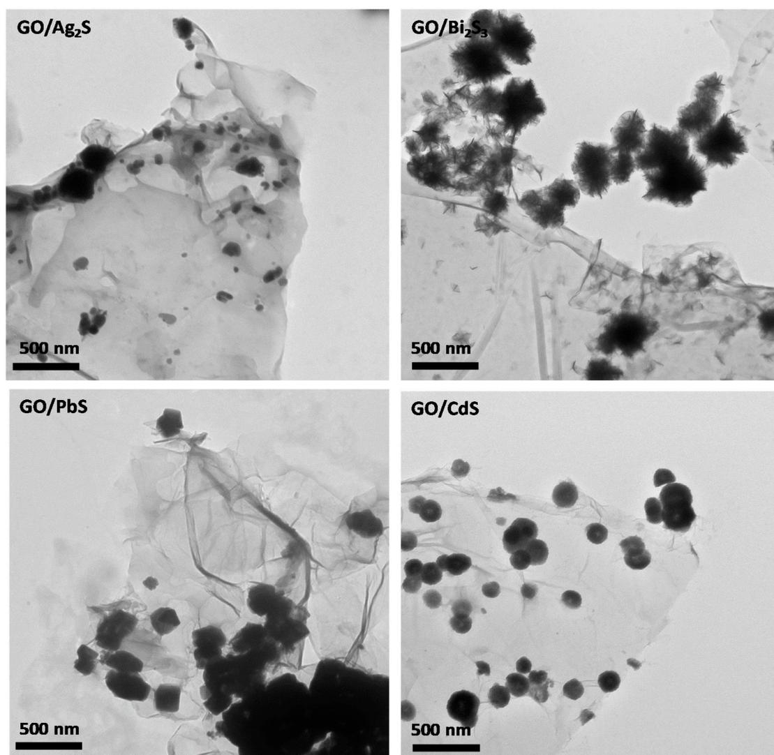
**Figure 3.** TEM images of graphene oxide hybrid nanostructures containing the metal sulfide nanophases indicated in the labels.
