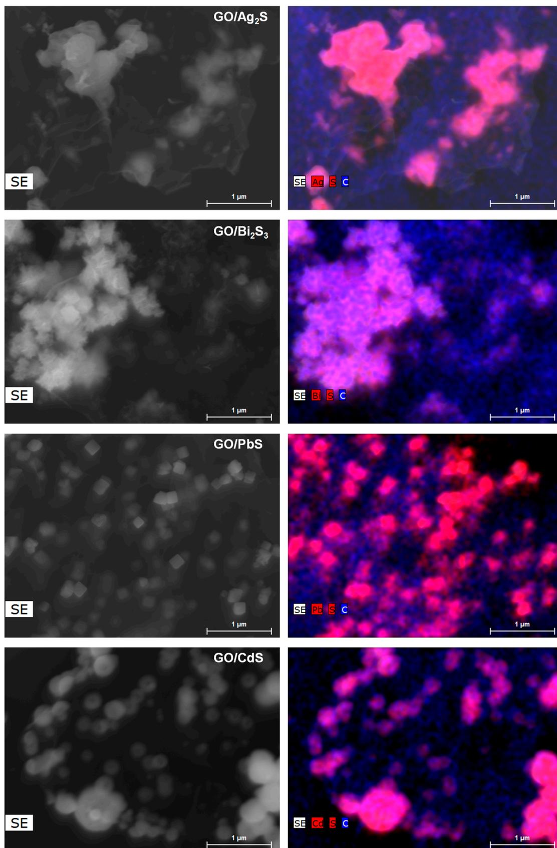
**Figure 4.** SEM images (left panel) and EDX mappings (right panel) of graphene oxide hybrid nanostructures containing metal sulfide nanophases.
