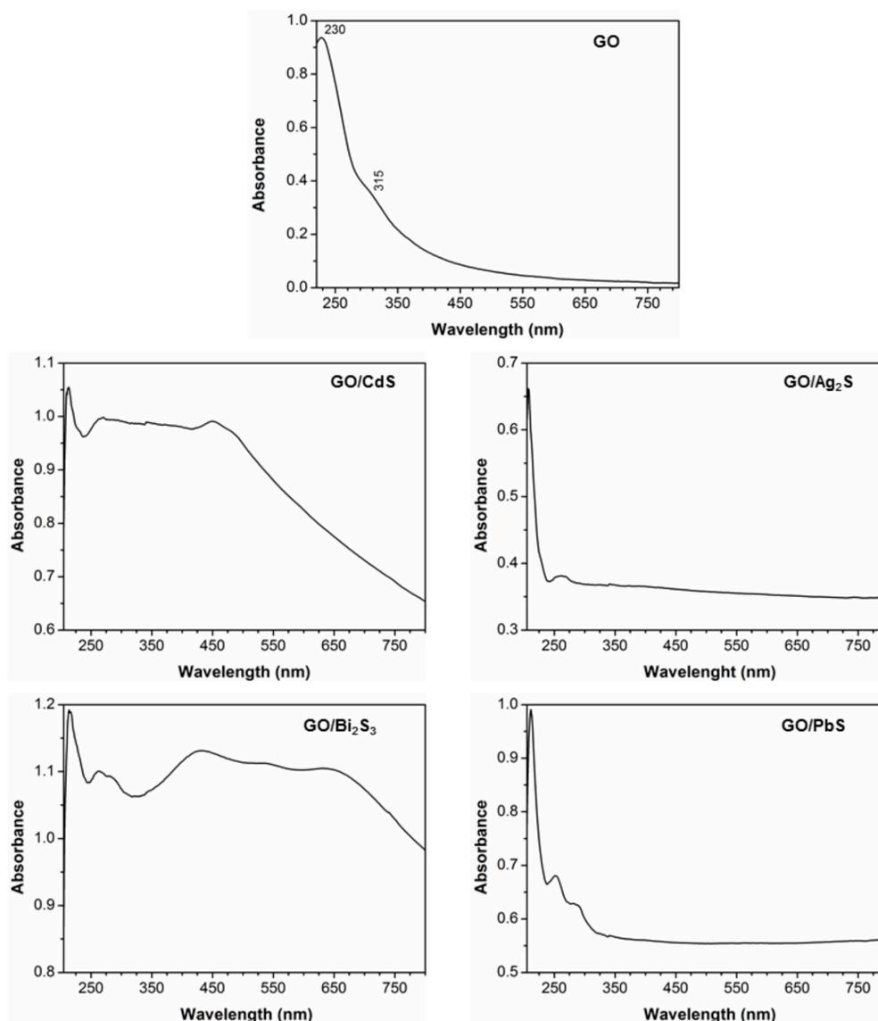
**Figure 2.** UV/Vis absorption spectra of ethanolic suspensions (0.05 mg/mL) of hybrid carbon nanostructures as indicated in the labels. For comparison, the UV/Vis spectrum of a graphene oxide suspension is also shown.
