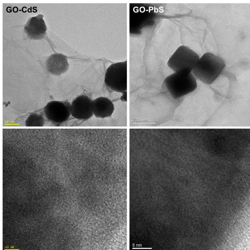
**Figure 5.** Graphene oxide (GO) sheets decorated with CdS and PbS nanophases: TEM images (**top**) and corresponding HRTEM images (**bottom**).
