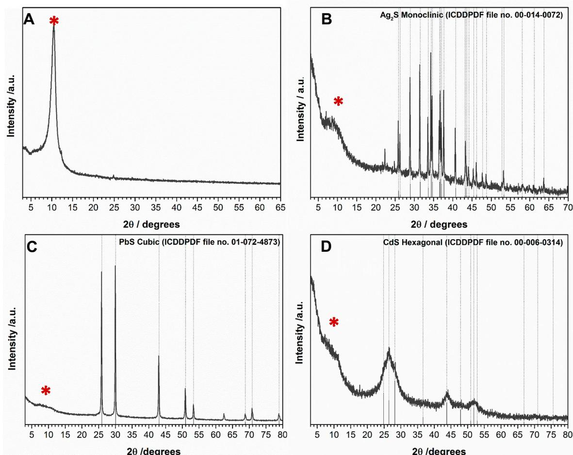
**Figure 1.** XRD patterns for (A) GO; (B) GO/Ag<sub>2</sub>S; (C) GO/PbS and (D) GO/CdS nanostructures. The vertical bars correspond to the diffractions peaks attributed to the respective metal sulfide. The diffraction peaks of GO are marked with \*.
