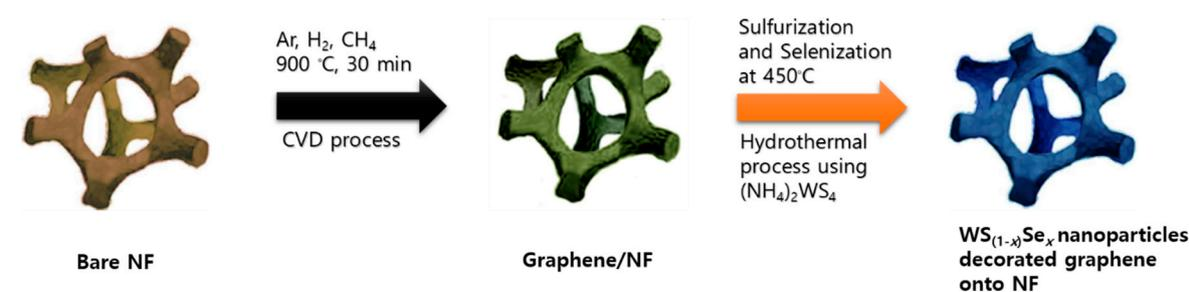
**Figure 1.** Schematic preparation process of graphene and the WS<sub>(1-x)</sub>Se<sub>x</sub>/graphene/NF catalyst.
