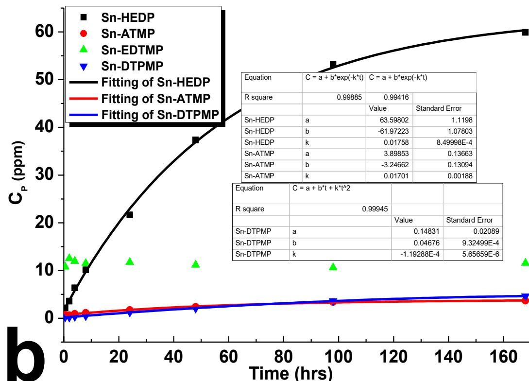
**Figure S5.** Empirical models that describe the leached elemental concentration ( $C$ ) as a function of time ( $t$ ) has been utilized to fit the dissolution kinetics of tin alkylphosphonates: (a) the fitting of tin
