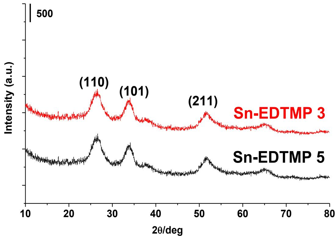
**Figure S7.** The wide-angle diffraction patterns of Sn-EDTMP
