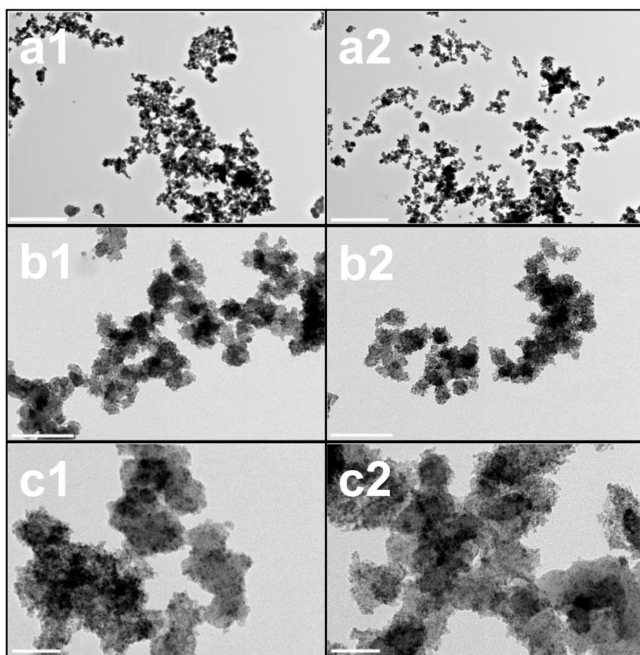
**Figure S1.** The HRTEM images of Sn-EDTMP 3. The scale bar of a, b, c are 1  $\mu$ m, 200 nm and 50 nm, respectively. The left, right column of images represents pristine and leached Sn-EDTMP 3, respectively.
