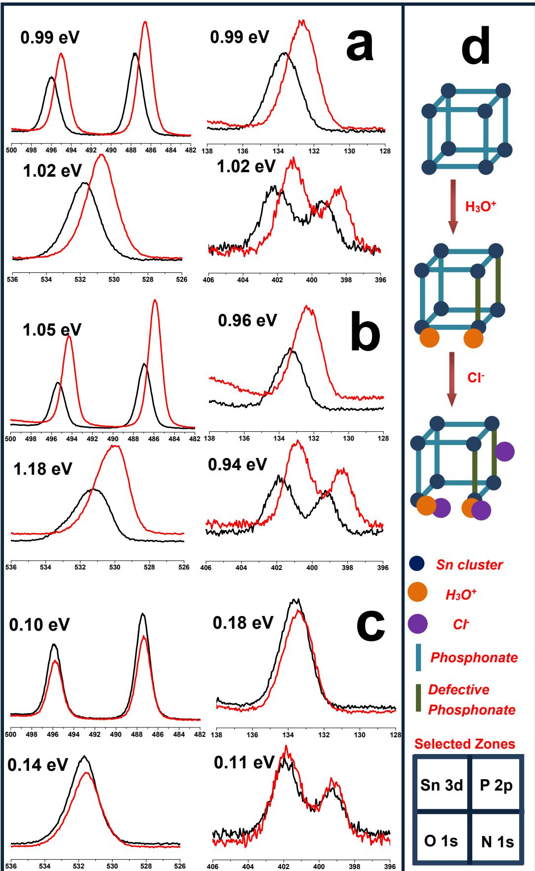
**Figure S3.** The selected XPS zones of pristine (black) and leached (red) tin alkylphosphonates: (a) Sn-ATMP; (b) Sn-EDTMP; (c) Sn-DTPMP. The structural breakdown of SnP in the presence of HCl is depicted as (d) to illustrate the formation of new species speculated from XPS spectra.
