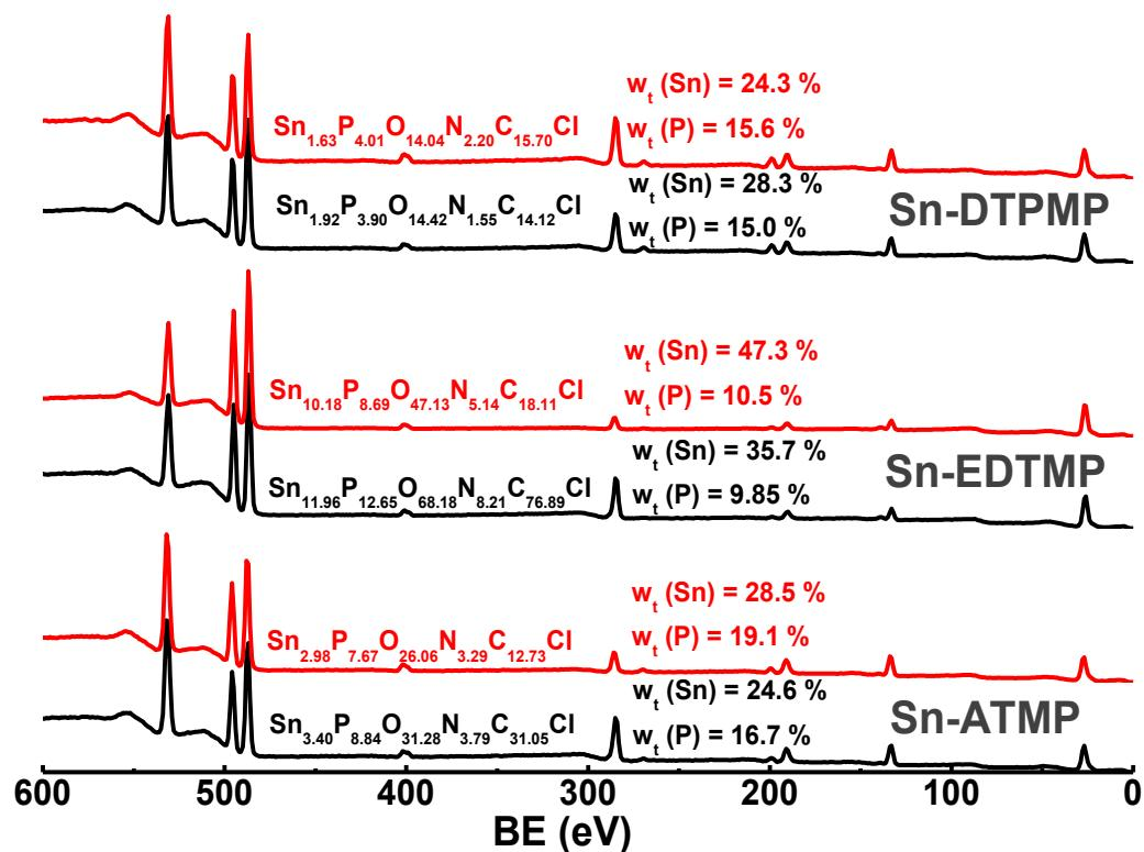
**Figure S2.** The XPS spectra of pristine (black) and leached (red) tin alkylphosphonates with tentative molecular formula. The weight percentages of tin, phosphorus before and after leaching are demonstrated for comparison.
