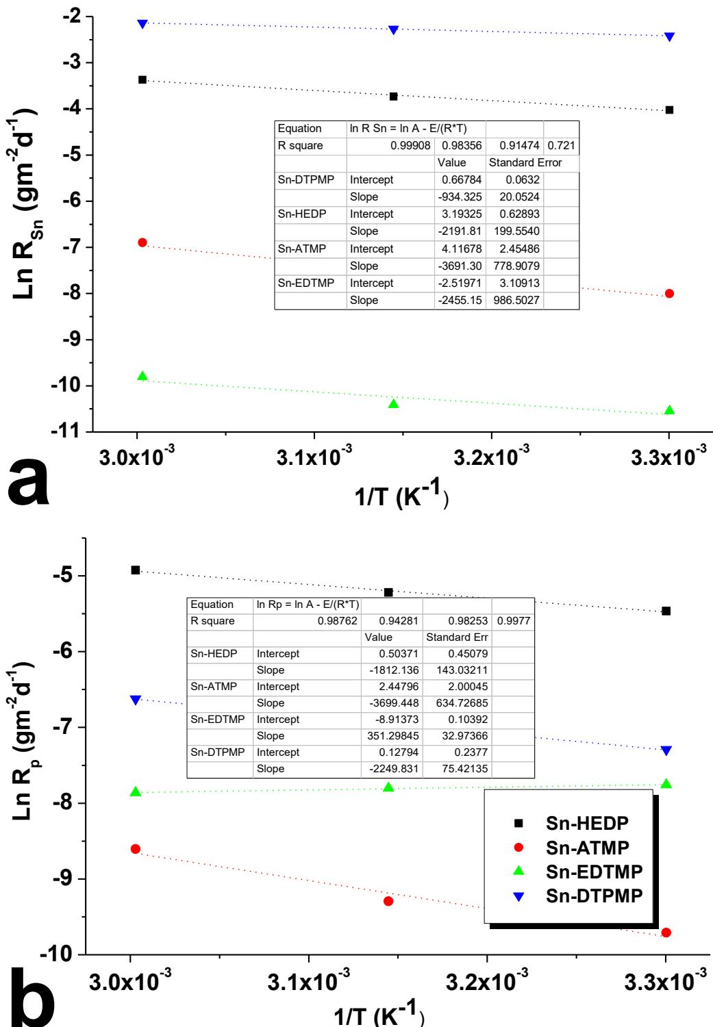
**Figure S6.** Temperature dependence of SnP dissolution rates and the variation of  $\ln R_i$  versus the
