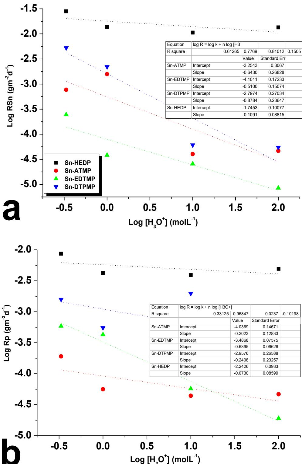
**Figure S4.** Acidity dependence of SnP dissolution rates and the variation of  $\log R_i$  versus the reciprocal acidity. The  $R_i$ ,  $k$ ,  $n$  represent the normalized dissolution rates, apparent normalized dissolution constant, partial order related to proton concentration, respectively. (a) tin; (b) phosphorus.
