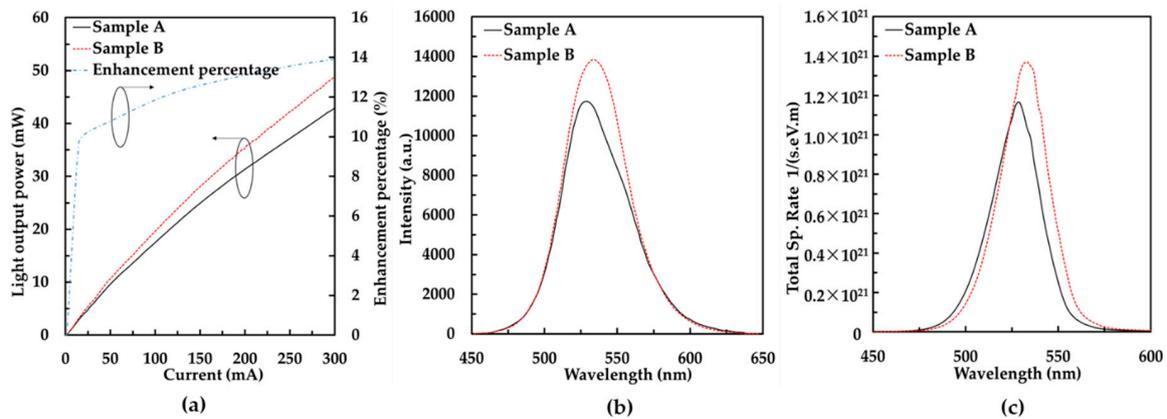
**Figure 3.** Light output properties of samples A and B: (a) measured light output power and enhancement percentage as a function of the injection current; (b) measured EL spectra at 300 mA; and (c) calculated EL spectra at 300 mA.
