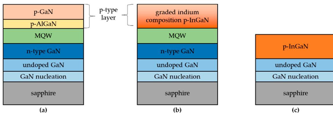
**Figure 1.** Schematic diagrams for the LED and p-InGaIn samples: (a) sample A; (b) sample B; and (c) sample C.
