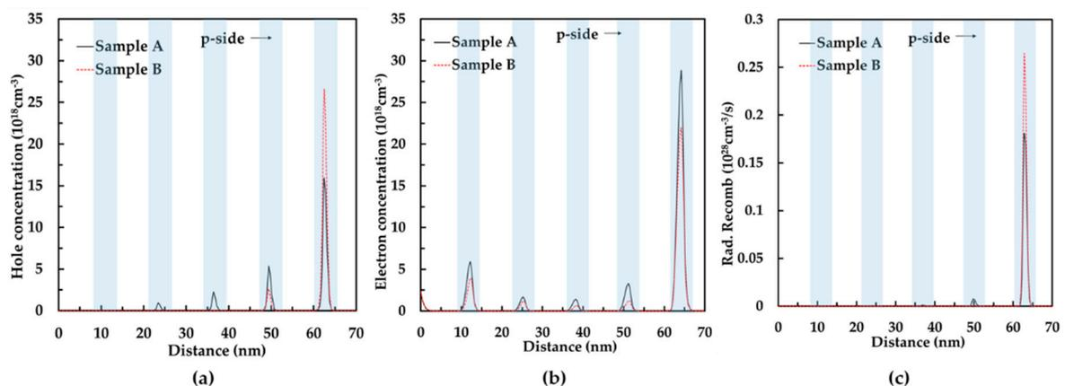
Figure 5. (a) Hole concentration distribution; (b) electron concentration distribution; and (c) radiation recombination rate distribution of samples A and B.
