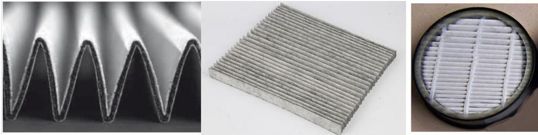
**Figure 12.** Example of folded filters that were made from a nonwoven bicotextile, PA-6 nanofibers filtration membrane, and adsorption textile (AT) sorption layer. The left is a cut of the folds, the middle is a view of the crimp material, and the right is tested filter.
