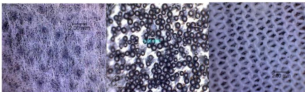
**Figure 6.** Chemviron Carbon ZORFLEX FM10, 100% woven activated carbon cloths from activated fibers.
