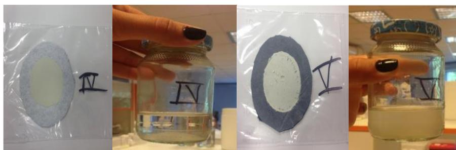
**Figure 11.** Examples of good and bad quality filtration for samples IV and V; 500 mL of water with 1% of a mixture solution was filtered through filter IV or V.
