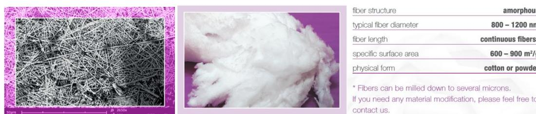
**Figure 4.** SEM image porous SiO<sub>2</sub> nanofibers, magnification 2650×, (left), wool from porous SiO<sub>2</sub> nanofibers (middle), and material characteristics (right).
