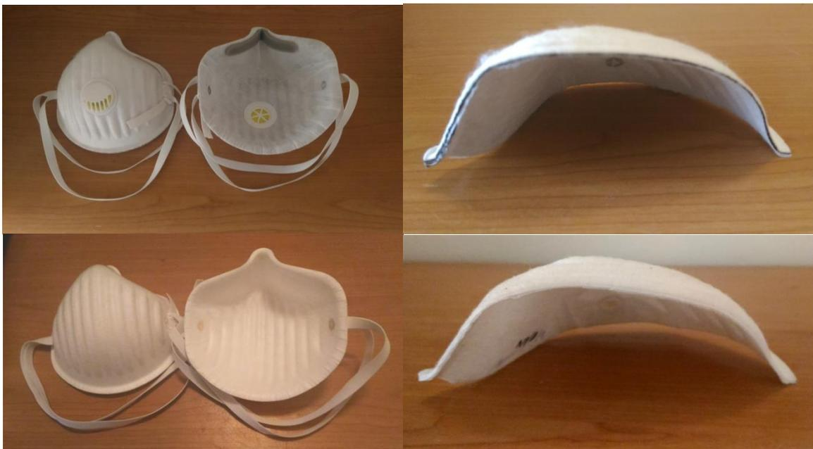
**Figure 13.** Example of respirators that were made with (**up**) and without (**down**) an adsorption layer. The left is the top and bottom view of the respirators (with or without valve). The right is a cut through of these respirators, with the view through the construction layer. From the top there is bicotextile, adsorption textile, nanofibers filtration membrane, and bicotextile.
