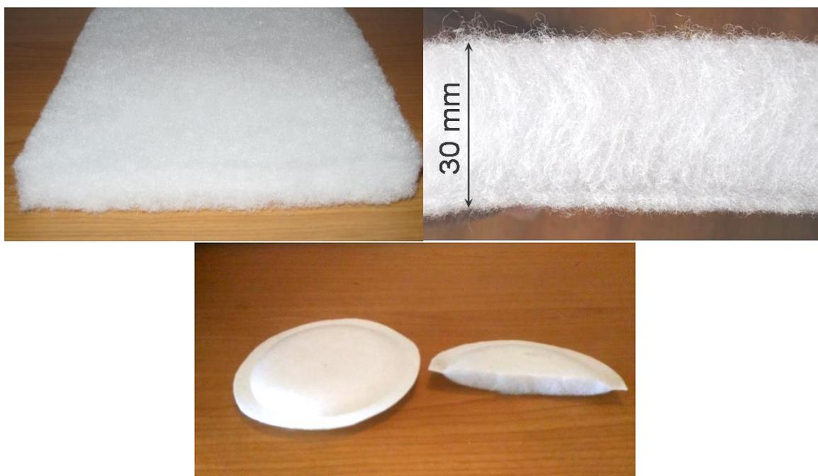
**Figure 14.** View on the cut of the struto textile, Elastic Universal, from JILANA, PLC, and the example of a filtration filler of the respirators made from struto textile and PVDF nanofibers membrane.
