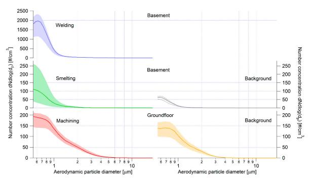
**Figure S2.** Particle number size distributions during welding, smelting, and machining (grinding and milling), and corresponding backgrounds measured by APS; solid line represents median for the measurement period and the corresponding shaded area shows interquartile span.
