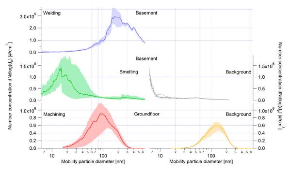
**Figure S1.** Particle number size distributions during welding, smelting, and machining (grinding and milling), and corresponding backgrounds measured by SMPS; solid line represents median for the measurement period and the corresponding shaded area shows interquartile span.
