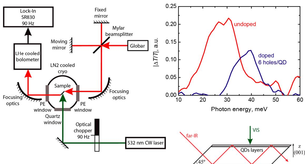
**Figure 3.** Experiment schematics and the measured spectra of the change of far-IR transmission due to external interband photoexcitation at 80 K. Data are plotted for undoped Ge/Si quantum dot structure (red curve) and doped structure (blue curve) with nominal doping of 6 holes/dot.
