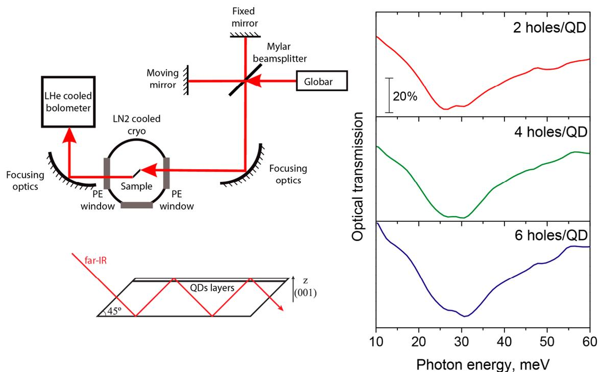
**Figure 2.** Experiment schematics and the measured far-IR transmission spectra of the Ge/Si quantum dot structures with different doping levels at 80 K. The labels at the curves indicate the nominal doping level.
