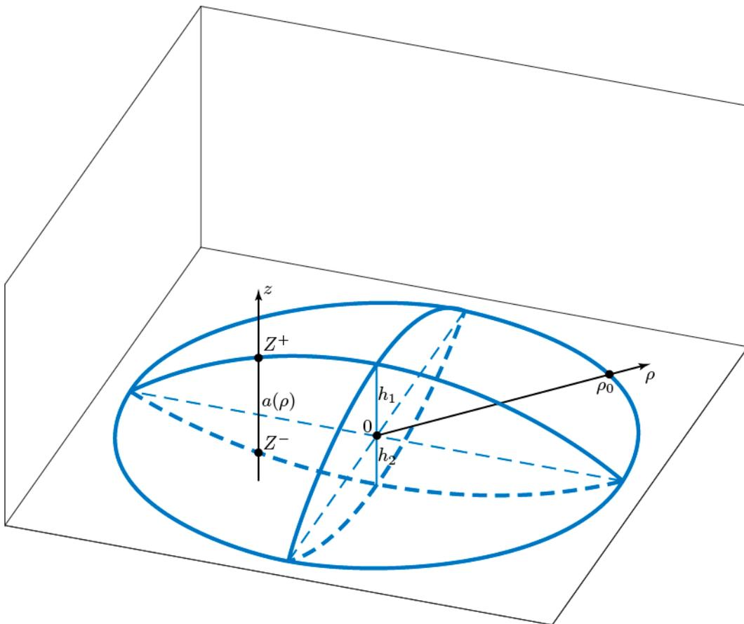
**Figure 1.** Schematics of the asymmetric biconvex quantum lens under consideration.
