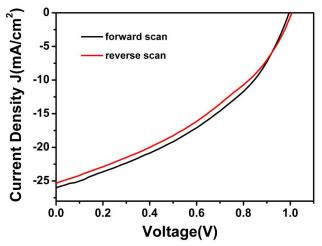
Fig S1. J-V curves of PSCs with DMSO-treated PEDOT:PSS layer (PVSK/DMSO/PVSK). The devices were scanned along the forward and reverse directions to study the hysteresis, with a delay time of 20 ms and a voltage step of 0.02 V s<sup>-1</sup>.
