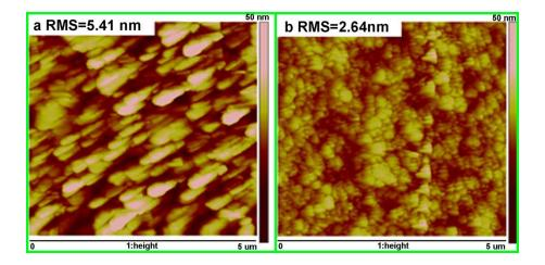
**Fig S2.** AFM image of (**a**) perovskite film processed on a pristine PEDOT:PSS film; (**b**) perovskite film processed on PEDOT:PSS film coated with the perovskite layer washing away by DMSO.
