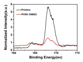
**Fig S3.** 2p XPS spectra of a pristine PEDOT:PSS film and PEDOT:PSS films treated with perovskite layer rinsed away with DMSO.
