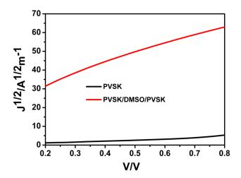
**Fig S4.** SCLC curves of devicess on a pristine PEDOT:PSS film (PVSK) and PEDOT:PSS films treated with perovskite layer rinsed away with DMSO (PVSK/DMSO/PVSK).
