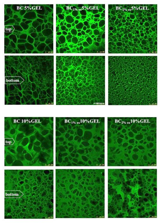
**Figure S1.** Confocal fluorescence microscopy images of BC–GEL membranes, without and with 5% and 10% GEL, and (non-, 1%, and 2%) oxidized BC. Top and bottom positions are relative to freezing plate position at freezing stage.
