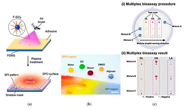
**Figure 7.** (a) Preparation of the SPO-SPI substrate; (b) Drop analysis of the SPO and SPI regions; (c) Demonstration of the SPO-SPI patterned substrate as a bioassay. Reprinted with permission from [49], with permission from American Chemical Society, 2019.
