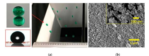
**Figure 6.** (a) WCA analysis; (b) SEM images of F-SiNPs coated solar mirrors. Reprinted with permission from [48], with permission from RSC Publishing, 2019.
