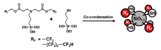
**Figure 2.** Fluorinated silica nanometer-sized particles synthesized by Mori et al. using a bottom-up method. Reprinted with permission from [34], with permission from Elsevier, 2019.
