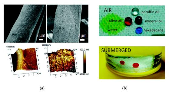
**Figure 5.** (a) SEM images (top) and AFM images (bottom) of the cotton fibers pre (left)- and post (right)-dip-coating; (b) Drop analysis with various oils and water in air (top) and submerged in water (bottom) of the dip-coated cotton fibers after 1000 abrasion cycles. Reprinted with permission from [47], with permission from RSC Publishing, 2019.
