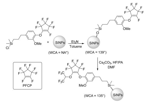
**Scheme 2.** Synthetic route employed by Jennings et al. for the synthesis of F-SiNPs. The structure of PFCP is shown in the inset. The WCA are also included. \* The bare particles were wet by water.
