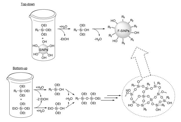
Scheme 1. General top-down and bottom-up methods used to obtain F-SiNPs.
