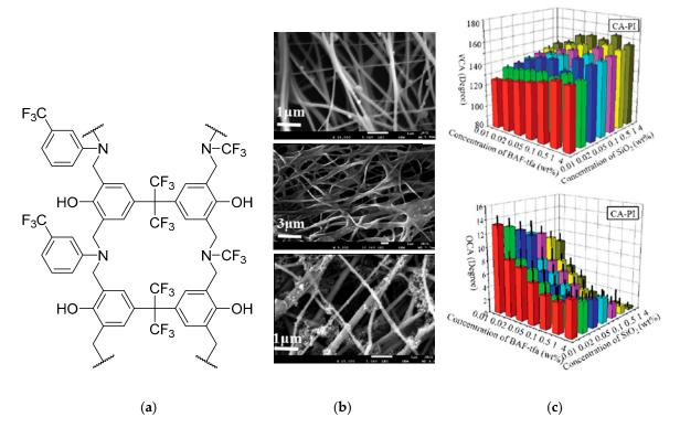
**Figure 9.** (a) BAF-tfa polymer used to functionalized SiNPs; (b) SEM images of CA-PI (top), CA-PI-BAF-tfa (middle), and CA-PI-BAF-tfa-SiNPs, and; (c) WCA (top) OLA (bottom) of membrane as a function of BAF-tfa and SiNPs concentration. Reprinted with permission from [57], with permission from RSC Publishing, 2019.
