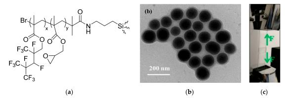
**Figure 4.** (a) Chemical structure of the functional group used to prepare F-SiNPs; (b) TEM images of the F-SiNPs; (c) Adhesive strength testing performed by He et al. Reprinted with permission from [46], with permission from American Chemical Society, 2019.
