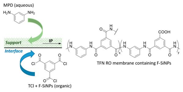
Scheme 5. Preparation of the polyamide TFN RO membrane containing F-SiNPs.
