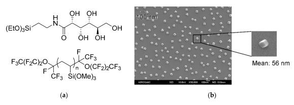
**Figure 8.** (a) Chemical structure of the reactive silanes used; (b) FE-SEM of the F-SiNPs prepared by Sawada and co-workers [50].
