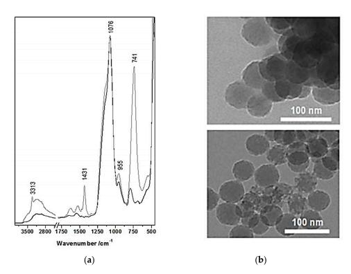
**Figure 3.** (a) DRIFT Spectrum of bare silica particles (black line) and fluorinated silica particles (grey line); (b) TEM images of bare silica particles (top) and fluorinated silica particles (bottom). Reprinted with permission from [36], with permission from RSC Publishing, 2019.
