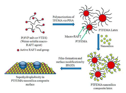
**Scheme 3.** Process used to prepare a superhydrophobic nanosilica composite. Reprinted with permission from [33], with permission from John Wiley and Sons, 2019.
