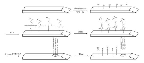
**Figure S2** Schematic diagram of the immobilization of the hapten conjugate 3-succinyl-CBF-OVA on the chip surface
