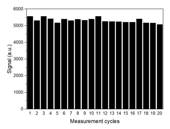
**Figure S3** Signal recovery after 20 cycles of measurements and regeneration with 0.5% SDS solution at pH = 1.9
