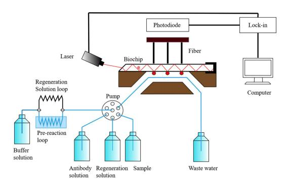
Figure S1 Schematic diagram of the optical waveguide-based fluorescent immunosensor
