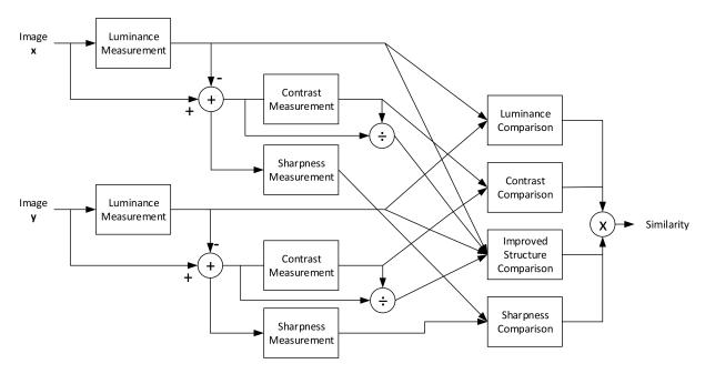
Figure 4. ISSIM-S diagram showing the measurement procedure.
