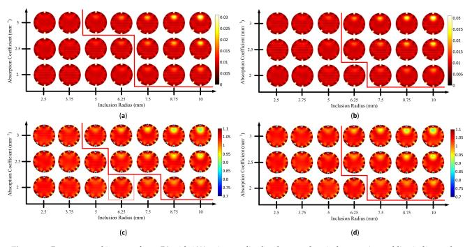
**Figure 20.** Reconstructed images of case B2 with 10% noise amplitude, phase, and optical properties; red line indicates the invisible (**left side**) and visible (**right side**) inclusions: (**a**)  $\mu_a$  MS-ISSIM-S, (**b**)  $\mu_a$  MOS, (**c**)  $\mu'_s$  MS-ISSIM-S, and (**d**)  $\mu'_s$  MOS.
