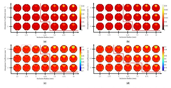
**Figure 19.** Reconstructed images of case B2 with 1% noise amplitude; red line indicates the invisible (**left side**) and visible (**right side**) inclusions: (**a**)  $\mu_a$  MS-ISSIM-S, (**b**)  $\mu_a$  MOS, (**c**)  $\mu'_s$  MS-ISSIM-S, and (**d**)  $\mu'_s$  MOS.
