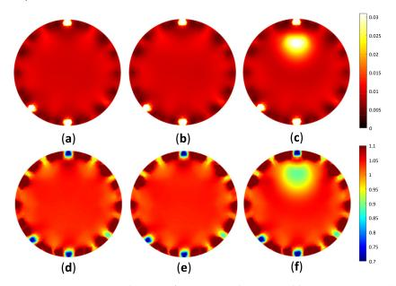
**Figure 10.** Reconstructed image of case A2, as shown in Table 1, representing (**a**)  $\mu_a$  homogeneous, (**b**)  $\mu_a$  invisible inclusion, (**c**)  $\mu_a$  visible inclusion, (**d**)  $\mu'_s$  homogeneous, (**e**)  $\mu'_s$  invisible inclusion, and (**f**)  $\mu'_s$  visible inclusion.
