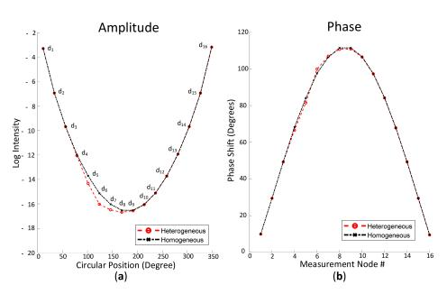
**Figure 8.** Obtained (**a**) light intensity and (**b**) phase shift from detectors attached around the model when  $S_1$  was used as the source with a red, dashed line, indicating heterogeneity, and black, dashed line for homogeneity.
