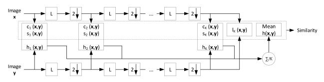
**Figure 5.** MS-ISSIM-S measurement procedure diagram. L denotes low-pass filtering and 2↓ refers to down-sampling by a factor of 2.
