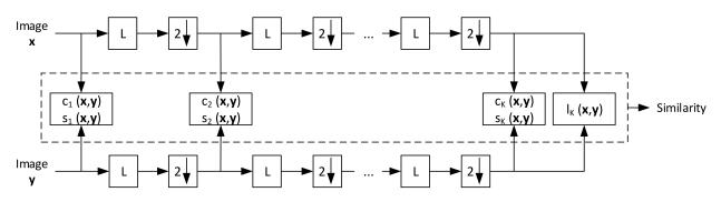
**Figure 3.** MS-SSIM diagram to demonstrate the measurement procedure. L denotes low-pass filtering and 2↓ refers to down-sampling by 2.
