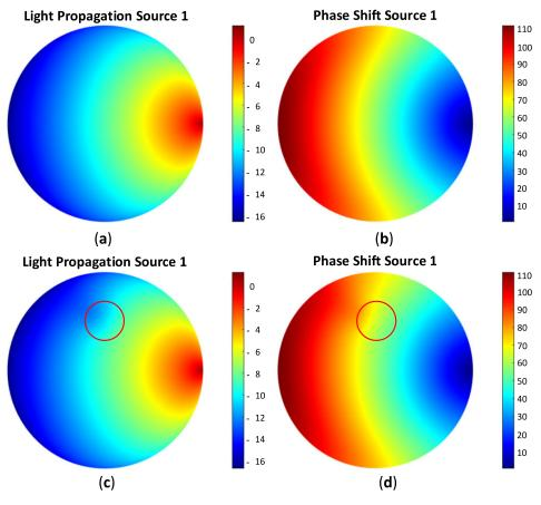
**Figure 7.** Distribution of (a) light propagation and (b) phase shift for homogeneous case; (c) light propagation and (d) phase shift for heterogeneous case, as in Figure 6b with the red circle, which shows the inclusion position when  $S_1$  was used as the source.
