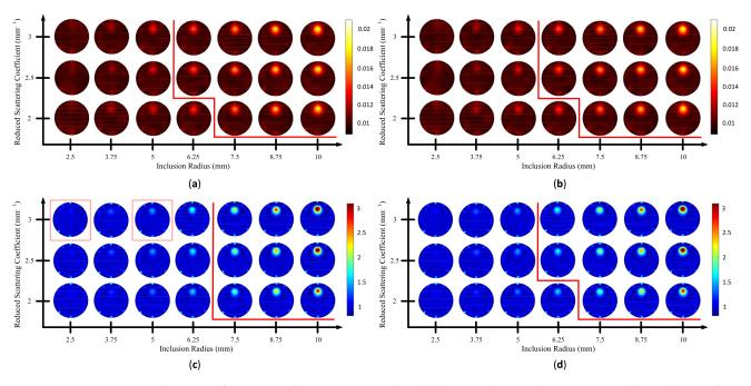
**Figure 18.** Reconstructed images of case B1 with 10% noise amplitude, phase, and optical properties; red line indicates the invisible (**left side**) and visible (**right side**) inclusions: (**a**)  $\mu_a$  MS-ISSIM-S, (**b**)  $\mu_a$  MOS, (**c**)  $\mu'_s$  MS-ISSIM-S, and (**d**)  $\mu'_s$  MOS.
