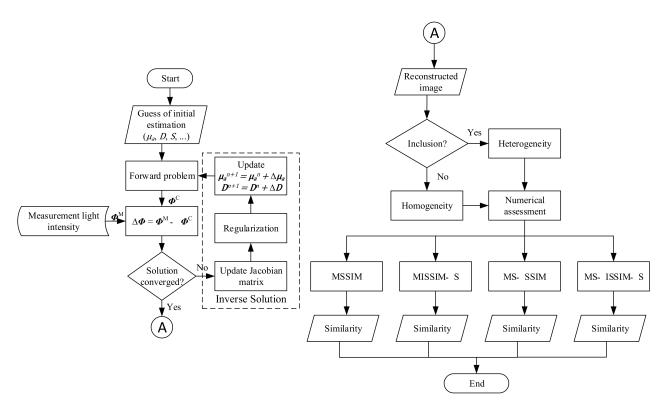
**Figure 1.** Block diagram of the process used to obtain similarity, where  $\mu_a$  and *D* are absorption and diffusion coefficients, respectively, *S* denotes the light source,  $\Phi^M$  expresses measured photon propagation, and  $\Phi^C$  is computed light from solving DE.
