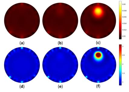
**Figure 9.** Reconstructed image of case A1, as shown in Table 1, representing (**a**)  $\mu_a$  homogeneous, (**b**)  $\mu_a$  invisible inclusion, (**c**)  $\mu_a$  visible inclusion, (**d**)  $\mu'_s$  homogeneous, (**e**)  $\mu'_s$  invisible inclusion, and (**f**)  $\mu'_s$  visible inclusion.
