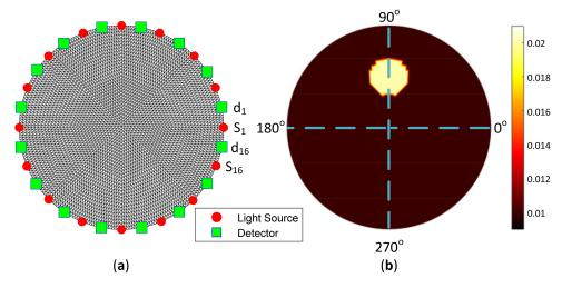
**Figure 6.** Model geometry showing (**a**) light sources (red dot) and detectors (green rectangle) where  $S_n$  is the *n* -th sensor and  $d_n$  denotes the *n* -th detector, as well as (**b**) artificial embedded inclusion position inside the tissue.
