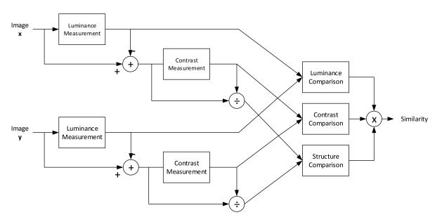
Figure 2. SSIM diagram to demonstrate the measurement procedure.
