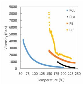
**Figure S1.** Plot showing the viscosities of four FDM-printable polymers—poly(caprolactone) (PCL), poly(lactic acid) (PLA), polyethylene (PE), poly(propylene) (PP)—with respect to the temperature.
