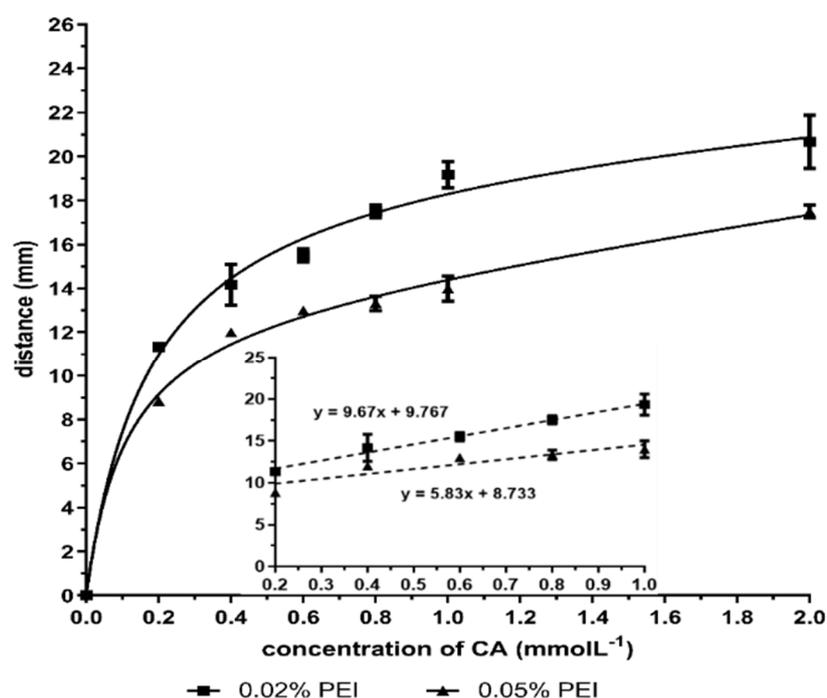
**Figure S1.** The proportional relationship between the color distance with the carminic acid (CA) concentration on the polyethyleneimine (PEI)-immobilized distance paper-based analytical device (dPAD) using PEI at the concentrations of 0.02% and 0.05% ( $n = 3$ ). Inset: Linear regression analysis and the best-fit line of CA between the ranges of 0.2 and 1.0  $\text{mmolL}^{-1}$ .
