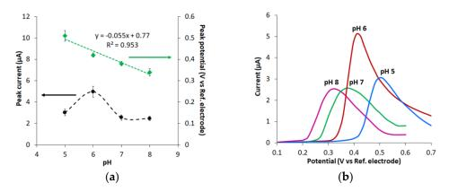
**Figure 5.** The effect of background electrolyte pH on UA oxidation peak current ( $I_p$ ) and peak potential ( $E_p$ ) on CVE<sub>act</sub> at 2.0 V (**a**); and the corresponding LS voltammograms for 0.01 mM UA in PB (**b**). Potential scan rate 0.05 Vs<sup>-1</sup>.
