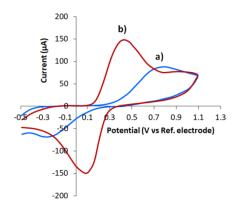
**Figure 3.** Cyclic voltammograms of 1.0 mM  $[Fe(CN)_6]^{4-}$  on CVE (**a**) and CVE<sub>act</sub> at 2.0 V (**b**) in 0.1 M KCl. Potential scan rate 0.05 Vs<sup>-1</sup>.
