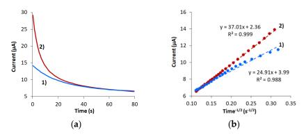
**Figure 4.** Chronoamperograms obtained at 0.5 V potential on CVE (1) and CVE<sub>act</sub> at 2.0 V (2) in 0.1 M KCl containing 1.0 mM K<sub>4</sub>[Fe(CN)<sub>6</sub>] (**a**). Dependencies  $i = f(t^{-1/2})$  are obtained from chronoamperograms on the corresponding electrodes (**b**).
