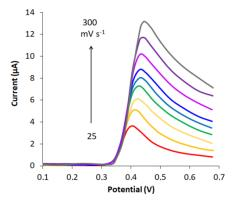
**Figure 6.** LS voltammograms of 0.01 mM UA on  $CVE_{act}$  at 2.0 V in PB pH 6 for different scan rates (25–300 mVs<sup>-1</sup>).
