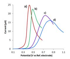
**Figure 1.** LS voltammograms of 0.1 mM UA for the CVE activated at 2.0 V (**a**), at 1.6 V (**b**) and at 1.0 V (**c**) and non-activated CVE (**d**) in PB pH 6.0. Potential scan rate  $0.05 \text{ Vs}^{-1}$ .
