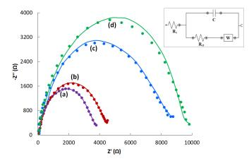
**Figure 2.** Experimental (points) and fitted (lines) Nyquist plots for  $\text{CVE}_{\text{act}}$  at 2.0 V (**a**), 1.6 V (**b**), 1.0 V (**c**) and CVE (**d**) in 0.1 M KCl containing 1.0 mM [Fe(CN)<sub>6</sub>]<sup>3-/4-</sup>. Insert: the diagram of an Randles equivalent cell.
