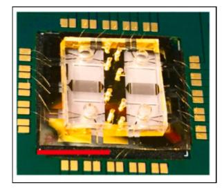
**Figure 5.** An ultra-high-frequency surface-acoustic-wave chip from Agostini et al. with the ability to multiplex up to four biomarkers. The red scale bar is 1 cm long. Reprinted with permission from [42]. Elsevier, 2021.
