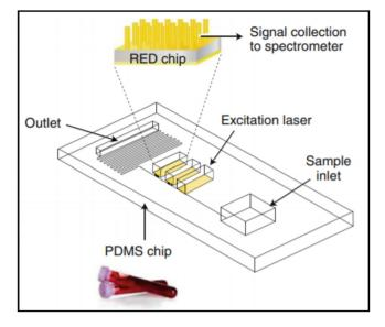
**Figure 4.** A SERS-based microfluidic device capable of a sample-in, results-out workflow from Rickard et al. Reprinted with permission from [48]. Springer Nature, 2020.
