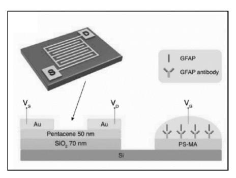
**Figure 2.** An organic field effect transistor (OFET) with an extended solution gate from Song et al. designed to measure GFAP. Reprinted with permission from [49]. John Wiley and Sons, 2017.
