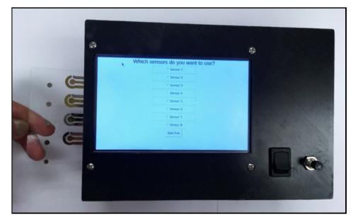
**Figure 1.** The μDrop system from Khetani et al. designed to perform differential pulse voltammetry to quantify C-tau and NF-L. Reprinted with permission from [36]. Elsevier 2021.
