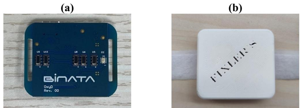
**Figure 3.** (a) The interior of the biochip, equipped with five photodetectors (PDs) and a single wavelength LED. (b) The chip inside its protective case.
