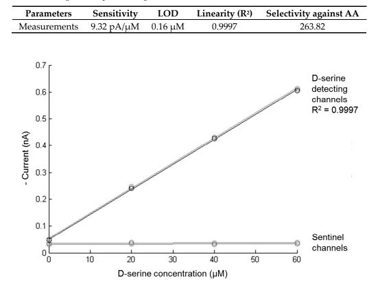
**Figure S2.** Linearity (R<sup>2</sup>) curve obtained from the calibration of the RgDAAO coated D-serine detecting MEA depicted in Figure 2.
