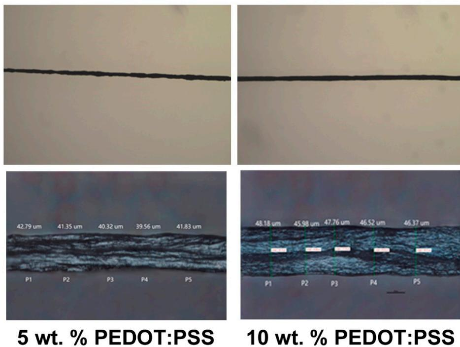
**Figure S3.** PEDOT:PSS fibers spun using different weight % of the dope solution with the same gauge needle.
