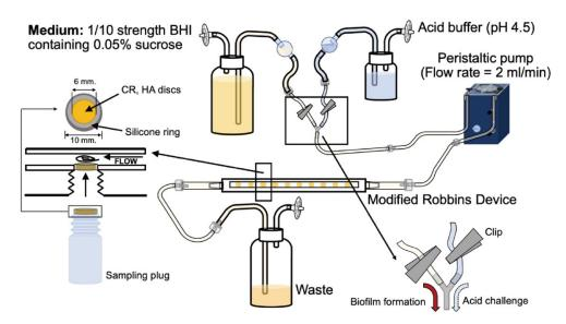
Figure 6. Modified Robbin device used in this study.
