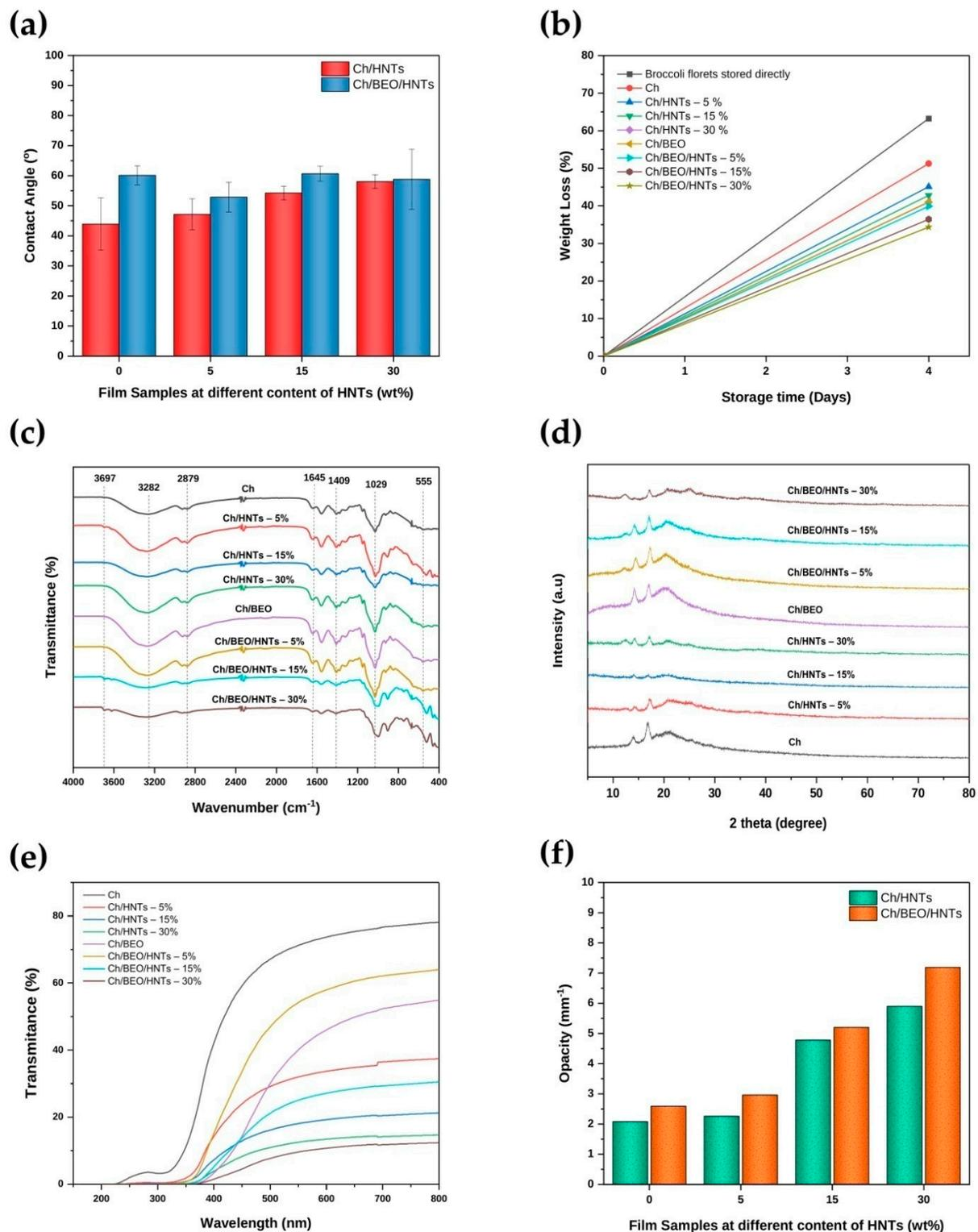
**Figure 7.** Figures representing the (a) contact angle of Ch films formulated with HNTs and BEO; (b) weight loss during 4 days storage; (c) ATR-FTIR spectrum of Ch films formulated with HNTs and BEO; (d) XRD pattern analysis of Ch films formulated with HNTs and BEO; (e) UV transmittance of Ch films formulated with HNTs and BEO; (f) opacity of Ch films formulated with HNTs and BEO.
