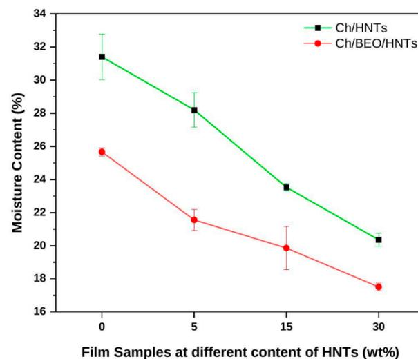
**Figure 3.** Moisture content of Ch films formulated with HNTs and BEO.
