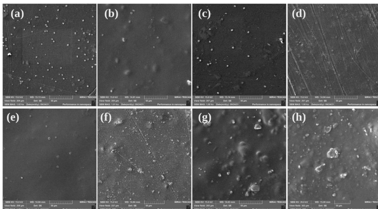
**Figure 6.** Scanning Electron Microscopy (SEM) images of the films. (a) Ch film; (b) Ch/HNTs—5%; (c) Ch/HNTs—15%; (d) Ch/HNTs—30%; (e) Ch/BEO; (f) Ch/BEO/HNTs—5%; (g) Ch/BEO/HNTs—15%; (h) Ch/BEO/HNTs—30%.
