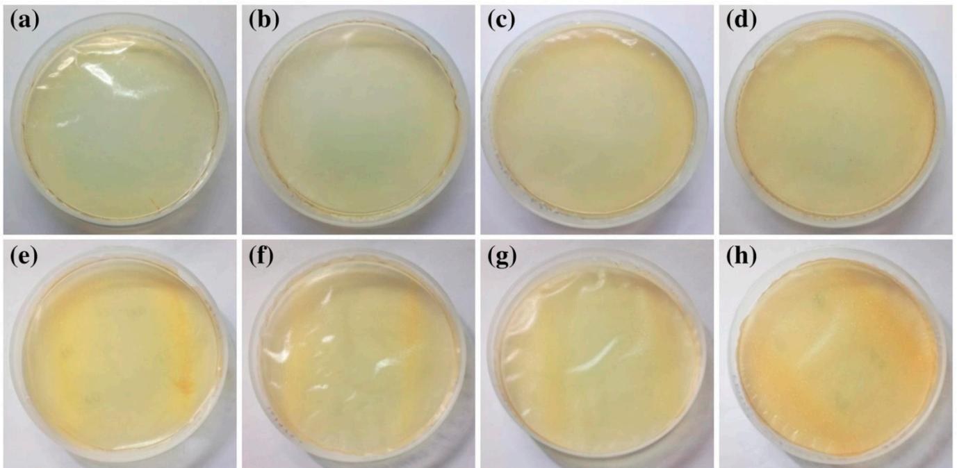
**Figure 2.** Representative images of nanocomposite films. (a) Ch film; (b) Ch/HNTs—5%; (c) Ch/HNTs—15%; (d) Ch/HNTs—30%; (e) Ch/BEO; (f) Ch/BEO/HNTs—5%; (g) Ch/BEO/HNTs—15%; (h) Ch/BEO/HNTs—30%.
