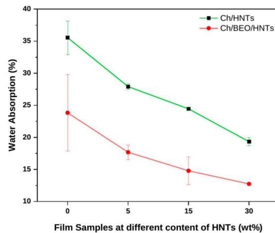
Figure 4. Water absorption of Ch films formulated with HNTs and BEO.
