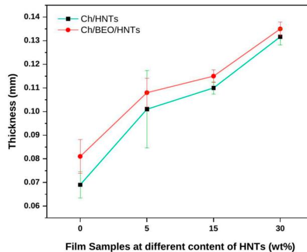
**Figure 1.** Thickness of Ch films formulated with HNTs and BEO.
