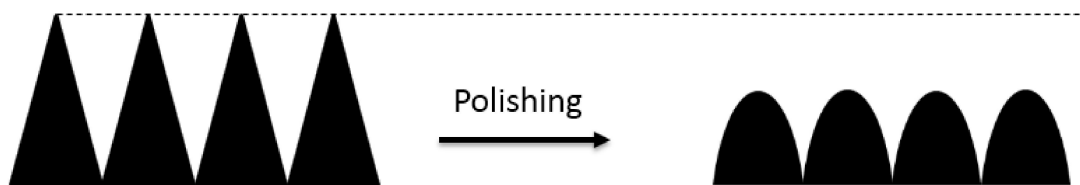
Figure 10. General polishing mechanisms.
