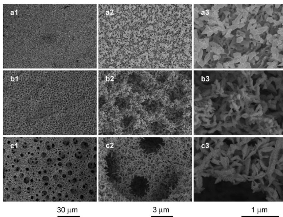
**Figure 4.** SEM images at different magnification scales for the PGF samples prepared using the technique of square-wave potential pulse in 2 M NaOH between the potential window of 0.8 and  $-5$  V for different times: (a1–a3) 100 s, (b1–b3) 3000 s, and (c1–c3) 12,000 s (adapted with permission from [33], copyright 2009 American Chemical Society).
