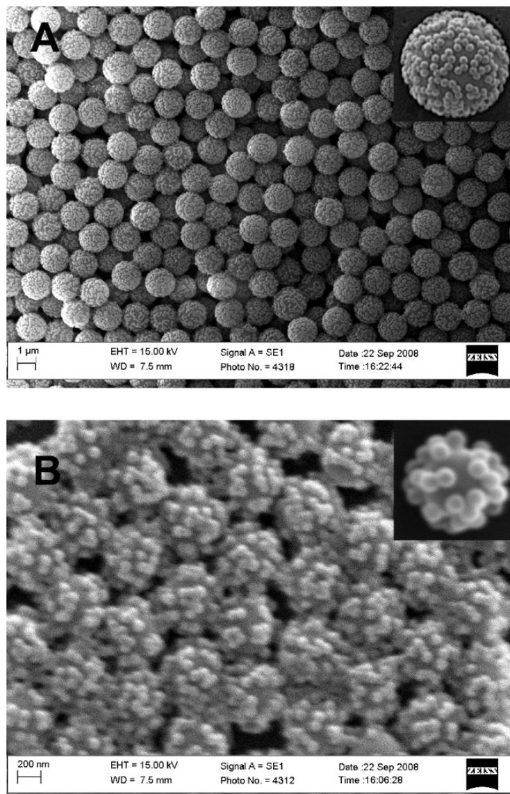
**Figure 5.** SEM images showing raspberry-like hierarchical templates prepared via coupling PS-COOH spheres with PH-NH<sub>2</sub>. Templates with (A) 1500/110 nm and (B) 450/80 nm core/satellite were prepared (reproduced with permission from [41], copyright 2010 American Chemical Society).
