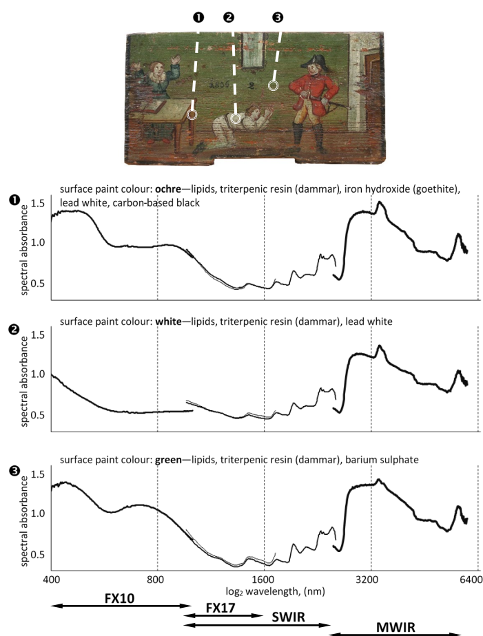
Figure 6. The specific regions of interest (ROIs) and the corresponding (average) spectra collected using the investigated hyperspectral cameras.
