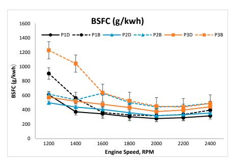
Figure 15. BSFC values at variable speeds.
