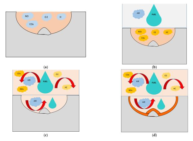
**Figure 10.** Staged combustion concept: (a) primary combustion, (b) introduction of subsequent fuel, (c) heated subsequent fuel and blend with previous traces product of combustion, (d) staged combustion of (c).
