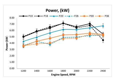
Figure 13. Power (kW) produced at various engine speeds.
