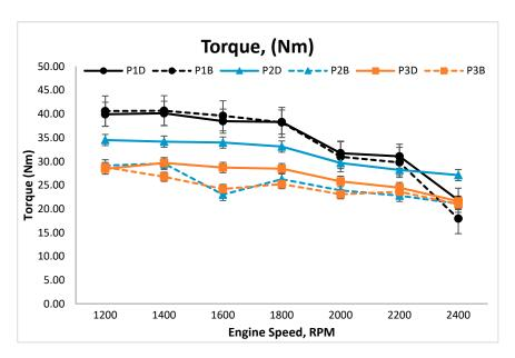
Figure 14. Torque (Nm) produced at variable speeds.
