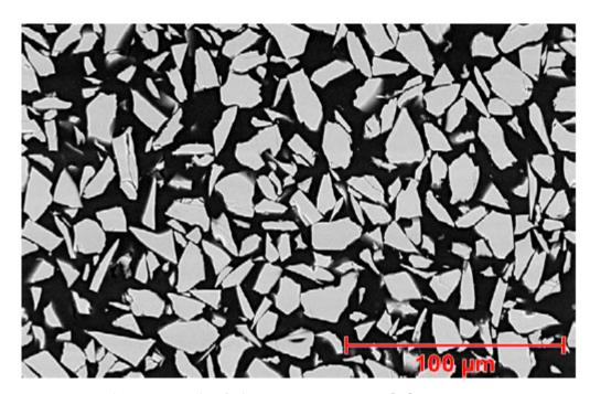
**Figure 6.** SEM photomicrographs of Al<sub>2</sub>O<sub>3</sub>·SiO<sub>2</sub> microstructure [22].
