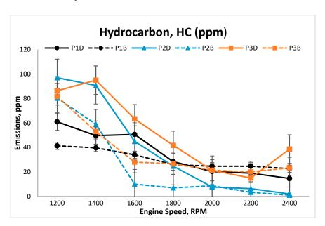
Figure 8. Hydrocarbon emissions at the variable engine speeds.
