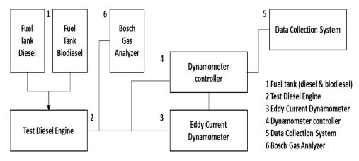
Figure 1. Schematic diagram for the experimental setup.
