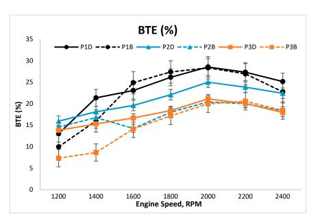
Figure 16. BTE percentage at variable engine speeds.
