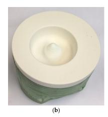
**Figure 4.** Piston coated with (a) YSZ and (b) Al<sub>2</sub>O<sub>3</sub>·SiO<sub>2</sub>.
