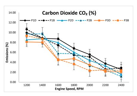
Figure 12. Carbon dioxide (CO<sub>2</sub>) emissions at variable speeds.
