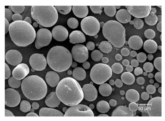
Figure 7. SEM photomicrographs (1000  $\times$  of magnification) of YSZ powder morphology [23].
