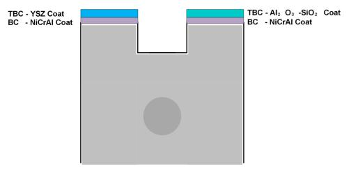
Figure 3. Thermal barrier coating layer on a piston.
