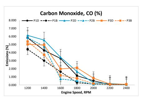
Figure 11. Carbon monoxide (CO) emissions at variable speeds.
