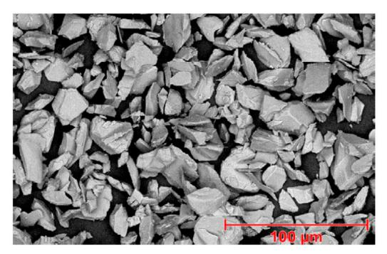
Figure 5. SEM photomicrographs (1000× of magnification) of Al<sub>2</sub>O<sub>3</sub>·SiO<sub>2</sub> powder morphology [22].
