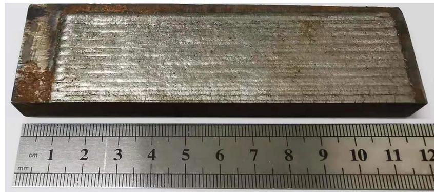
**Figure 1.** Macroscopic morphology of the Co-based alloy coating fabricated via the laser cladding process.
