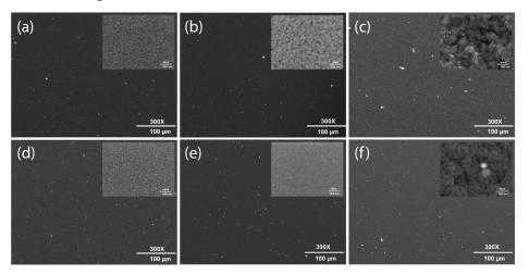
**Figure 7.** SEM data for Zr thin films deposited with fluence  $0.52 \text{ J/cm}^2$  and a wavelength of 532 nm and substrate temperatures of (a)  $25 \,^{\circ}\text{C}$ , (b)  $300 \,^{\circ}\text{C}$ , and (c)  $500 \,^{\circ}\text{C}$ , and with a wavelength of  $1064 \, \text{nm}$  and substrate temperatures of (d)  $25 \,^{\circ}\text{C}$ , (e)  $300 \,^{\circ}\text{C}$ , and (f)  $500 \,^{\circ}\text{C}$ .
