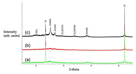
**Figure 2.** XRD data for Zr thin films deposited with a wavelength of 1064 nm, fluences of (a)  $0.26 \text{ J/cm}^2$ , (b)  $0.52 \text{ J/cm}^2$ , and (c)  $1.04 \text{ J/cm}^2$ , and substrate temperature of  $500 \,^{\circ}\text{C}$ .
