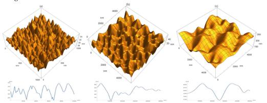
**Figure 9.** Computational results. Surface morphology is shown after 1 hr of film growth at substrate temperatures of (a)  $25 \,^{\circ}$ C, (b)  $300 \,^{\circ}$ C, and (c)  $500 \,^{\circ}$ C. Note that the scale along the x and y axes in the panel (a) is five times smaller than in the panels (b,c).
