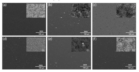
**Figure 5.** SEM data for Zr thin films deposited with a wavelength of 532 nm, fluences (**a**)  $0.26 \text{ J/cm}^2$ , (**b**)  $0.52 \text{ J/cm}^2$ , and (**c**)  $1.04 \text{ J/cm}^2$ , and substrate temperature of  $500 \,^{\circ}$ C, and with a wavelength of 1064 nm and fluences of (**d**)  $0.26 \text{ J/cm}^2$ , (**e**)  $0.52 \text{ J/cm}^2$ , and (**f**)  $1.04 \text{ J/cm}^2$ .
