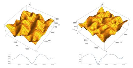
**Figure 10.** Computational results. Surface morphology is shown after 1 hr of film growth at a substrate temperature of 500  $^{\circ}$ C. The atomic flux *F* in the panel (**b**) is 25% higher than in the panel (**a**).
