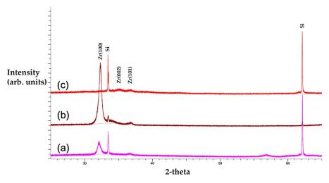
**Figure 4.** XRD data for Zr thin films deposited with wavelength of 1064 nm, fluence  $0.52 \, \text{J/cm}^2$ , and substrate temperatures of (a)  $25 \, ^{\circ}\text{C}$ , (b)  $300 \, ^{\circ}\text{C}$ , (c)  $500 \, ^{\circ}\text{C}$ .
