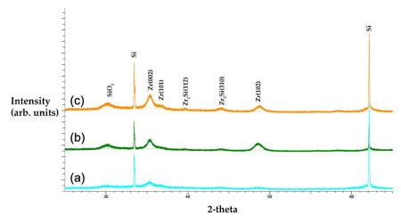
**Figure 1.** XRD data for Zr thin films deposited with a wavelength of 532 nm, fluences of (a)  $0.26 \,\text{J/cm}^2$ , (b)  $0.52 \,\text{J/cm}^2$ , and (c)  $1.04 \,\text{J/cm}^2$ , and substrate temperature of  $500 \,^{\circ}\text{C}$ .
