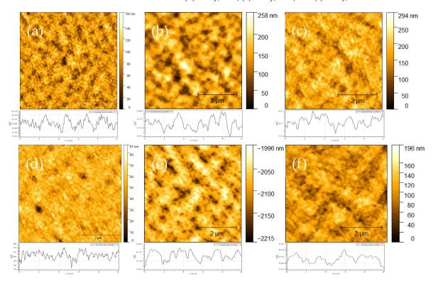
**Figure 6.** AFM data for Zr thin films deposited with a wavelength of 532 nm, fluences (a)  $0.26 \, \text{J/cm}^2$ , (b)  $0.52 \, \text{J/cm}^2$ , and (c)  $1.04 \, \text{J/cm}^2$ , and substrate temperature of  $500 \, ^{\circ}\text{C}$ , and with a wavelength of  $1064 \, \text{nm}$ , fluences of (d)  $0.26 \, \text{J/cm}^2$ , (e)  $0.52 \, \text{J/cm}^2$ , and (f)  $1.04 \, \text{J/cm}^2$ , and substrate temperature of  $500 \, ^{\circ}\text{C}$ .
