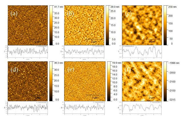
**Figure 8.** AFM data for Zr thin films deposited with a wavelength of 532 nm, fluence  $0.52 \text{ J/cm}^2$ , and substrate temperatures of (a)  $25 \,^{\circ}\text{C}$ , (b)  $300 \,^{\circ}\text{C}$ , and (c)  $500 \,^{\circ}\text{C}$ , and a wavelength of  $1064 \, \text{nm}$ , fluence  $0.52 \, \text{J/cm}^2$ , and substrate temperatures of (d)  $25 \,^{\circ}\text{C}$ , (e)  $300 \,^{\circ}\text{C}$ , and (f)  $500 \,^{\circ}\text{C}$ .
