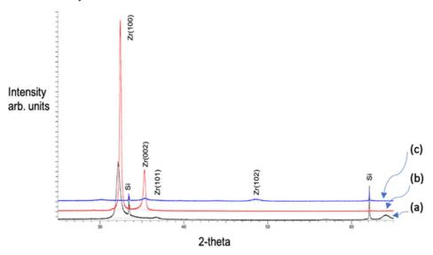
**Figure 3.** XRD data for Zr thin films deposited with a wavelength of 532 nm, fluence of  $0.52 \text{ J/cm}^2$ , and substrate temperatures of (a)  $25 \,^{\circ}\text{C}$ , (b)  $300 \,^{\circ}\text{C}$ , and (c)  $500 \,^{\circ}\text{C}$ .
