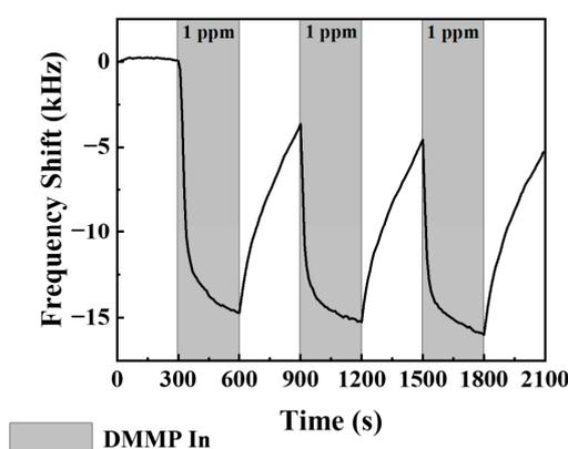
**Figure 9.** The repeatability of the SAW sensor at a DMMP concentration of 1 ppm.
