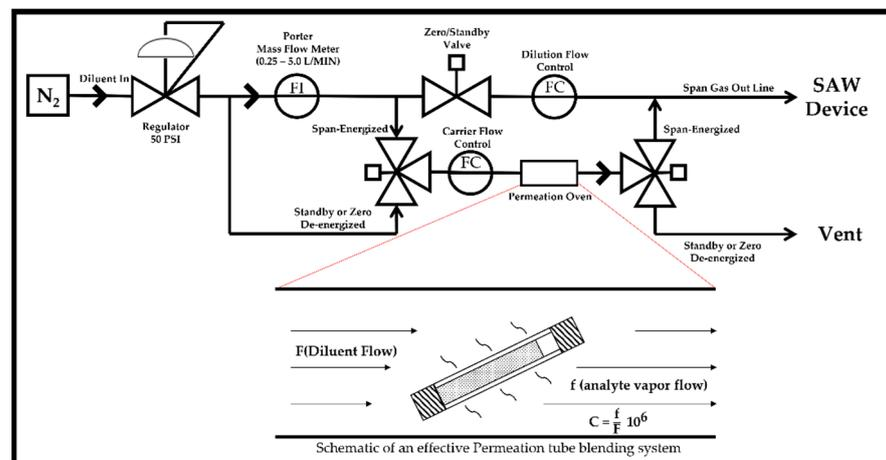
**Figure 6.** Gas feeding system: Base Module Flow Diagram for the permeation tube and schematic of and effective permeation tube blending system from KIN-TEK [37,38].
