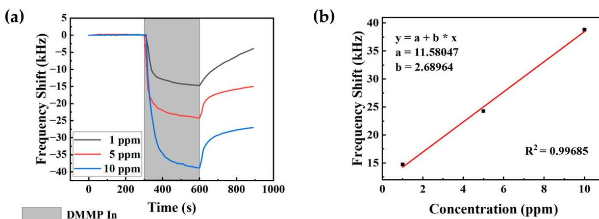
**Figure 8.** DMMP response from SAW sensors with PSS-TU3. (a) DMMP experiments at various concentrations. (b) Linearity according to DMMP reaction of various concentrations.
