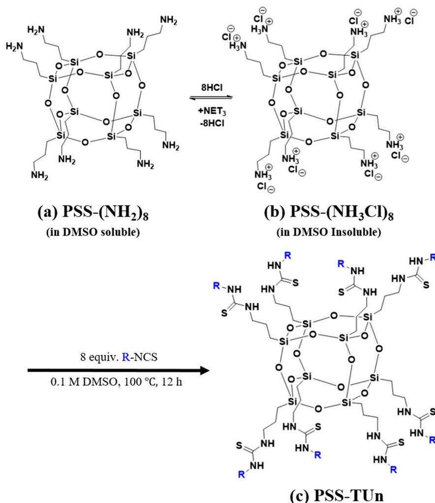
**Figure 3.** Schematic illustration of the synthesis process and each structure: (a) PSS-(NH<sub>2</sub>)<sub>8</sub>, (b) PSS-(NH<sub>3</sub>Cl)<sub>8</sub>, (c) PSS-TU<sub>n</sub> ( $n = 1, 2, 3$ ).
