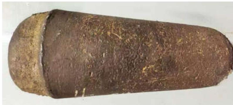
**Figure 1.** Image of ingot prepared by induction vacuum furnace.
