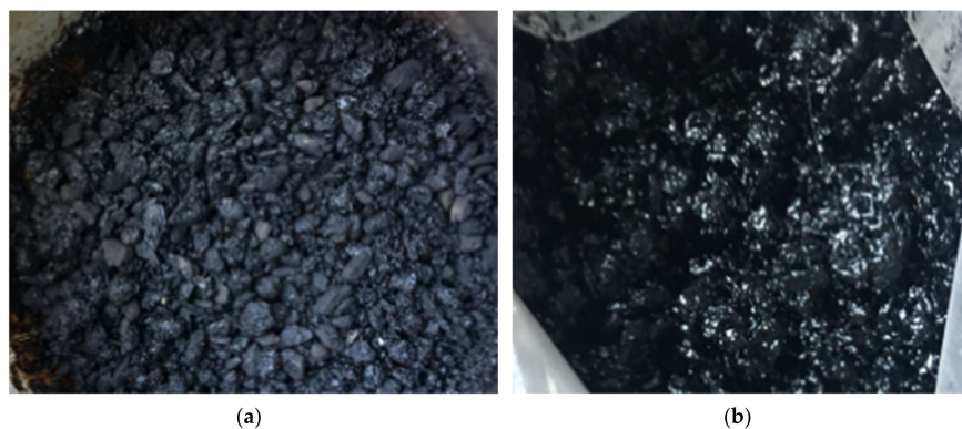
Figure 10. Appearance of OSW and stone after asphalt adsorption capacity test. (a) OSW; (b) stone.
