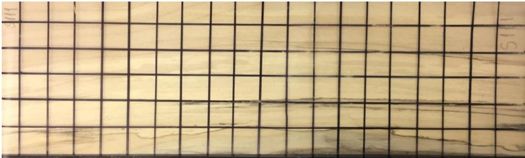
**Figure 1.** Acetate template on the surface of the wood specimen used to sort spalted wood samples.
